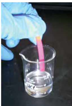
Figure 1 The pH of hydrochloric acid is tested with litmus paper. (credit: David Berardan)
