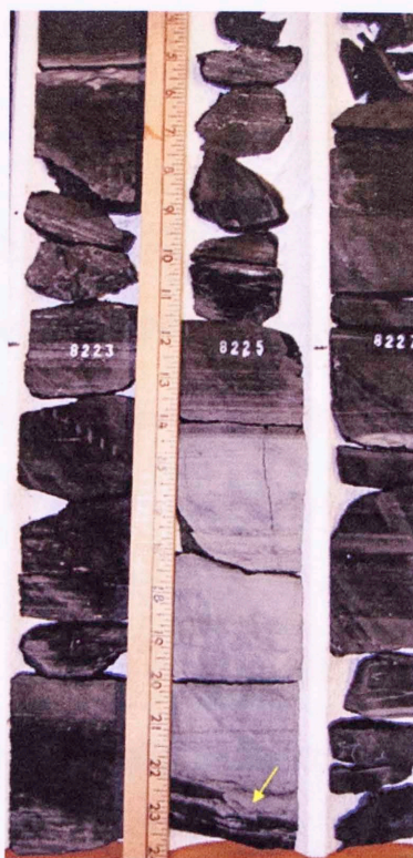
Figure 4.28. Core photograph displaying the debris flow deposit in John Porter #3 well at 8225 ft. (2506.9 m) to 8226 ft. (2507.3 m). The arrow marks the platy clast at the base of the deposit.
