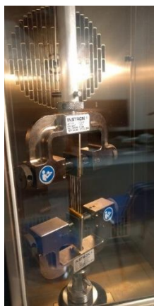
Figure 5.2 Fiber stretching process (5 mm/min strain rate and in 135°C Instron 5969 environmental chamber).
