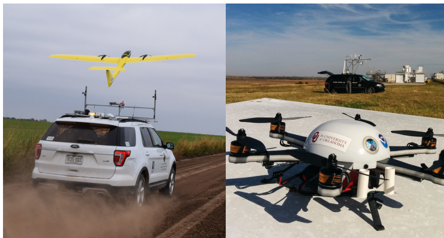
Figure 5.2: CU TTWistor launching from the roof of a chase vehicle (left). The Meteomatics Meteodrone hexacopter (right). These platforms, along with the OU CopterSonde, were the primary methods of sampling the PBL during EPIC.
