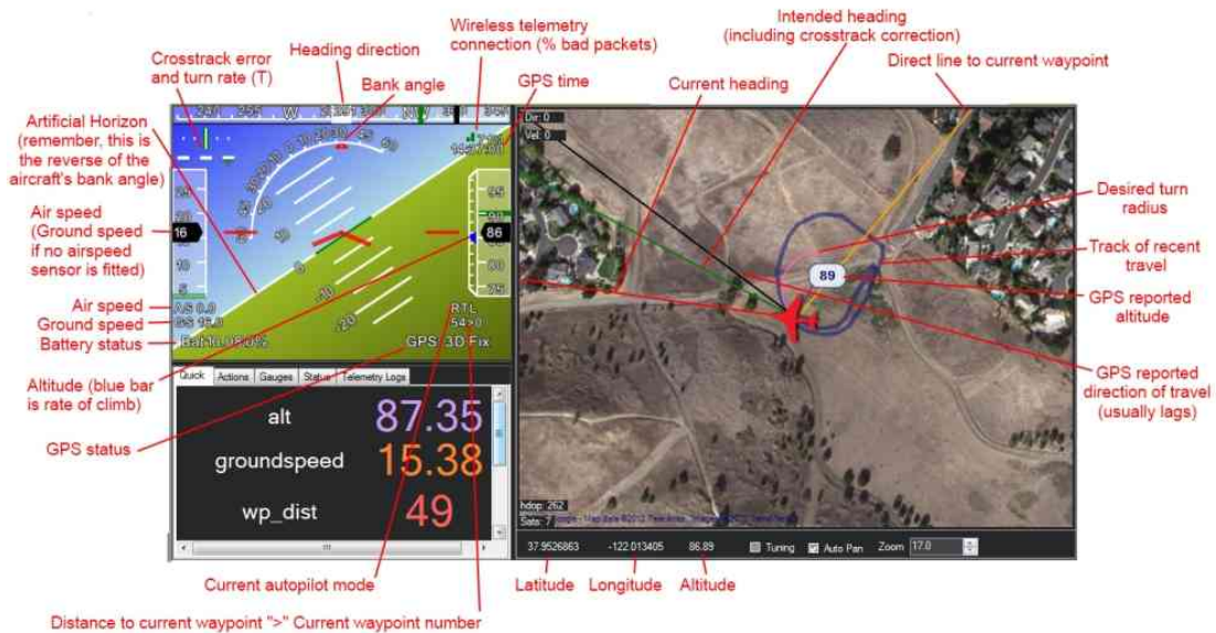
Figure 2.2: Heads Up Display (HUD) screen in Mission Planner ( http://ardupilot.org/planner/docs/mission-planner-ground-control-station.html ). This screen provides information about an aircraft when connected to the ground station, including heading, battery voltage, altitude, and ground speed. This software can also be used to build flight missions and perform other diagnostics.
