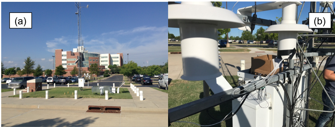
Figure 3.8: (a) The Mesonet tower in the parking lot of the National Weather Center in Norman, Oklahoma. (b) Mounted on the tower are two aspirated chambers as reference in calibrating the iMet temperature and humidity sensors.
