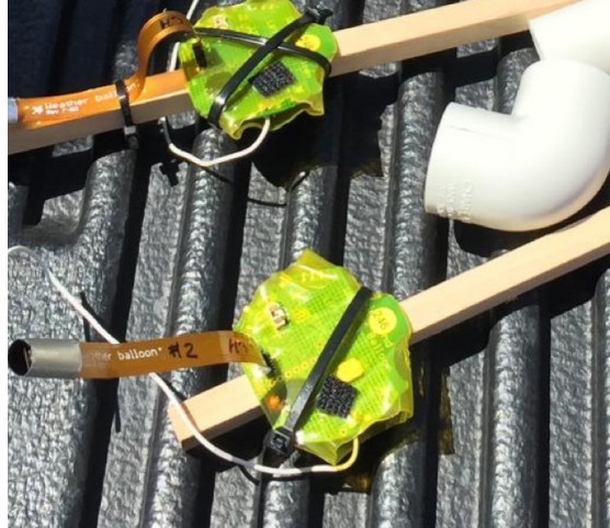
Figure 2.3: Windsond by Sparv Embedded. These thermodynamic sensors are only a few centimeters in size, making them ideal for mounting onto a UAV or releasing with a small balloon. Shown here are two packages mounted to wooden dowels, which was one of the various methods of integrating with a rwUAS.
