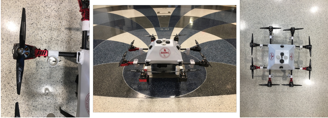
Figure 1.5: The CopterSonde, an octo-rotor UAS designed and built by CASS at OU. This first-generation CopterSonde has been the primary mode of testing sensor placement and responses along with collecting atmospheric data since May 2017.
