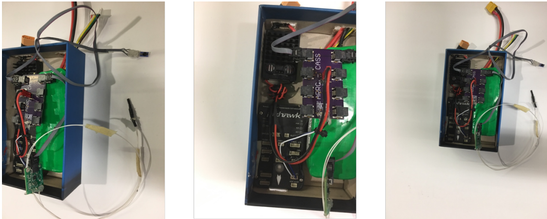
Figure 2.6: The iMet-XF sensor package fully integrated with a Pixhawk autopilot. This setup allowed for total onboard synchronization and streaming of a single output to the ground station.
