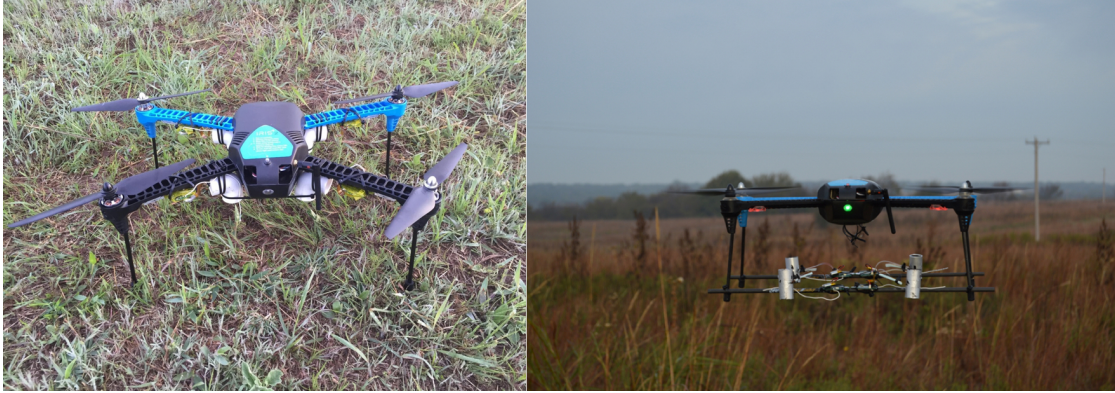
Figure 2.4: The Iris+ by 3D Robotics is a quadcopter controlled by a Pixhawk autopilot and served as one of the primary experimental platforms for atmospheric research at CASS for several years. Numerous iterations of sensor placement of the Windsond probes were evaluated during this time when it was determined that response characteristics were impacted by location.
