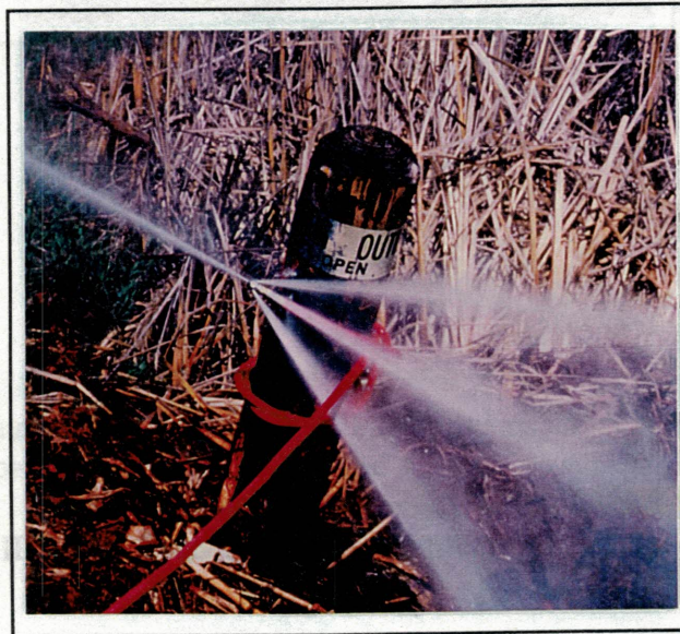
Figure 22 Jetting action of a thruster head.
