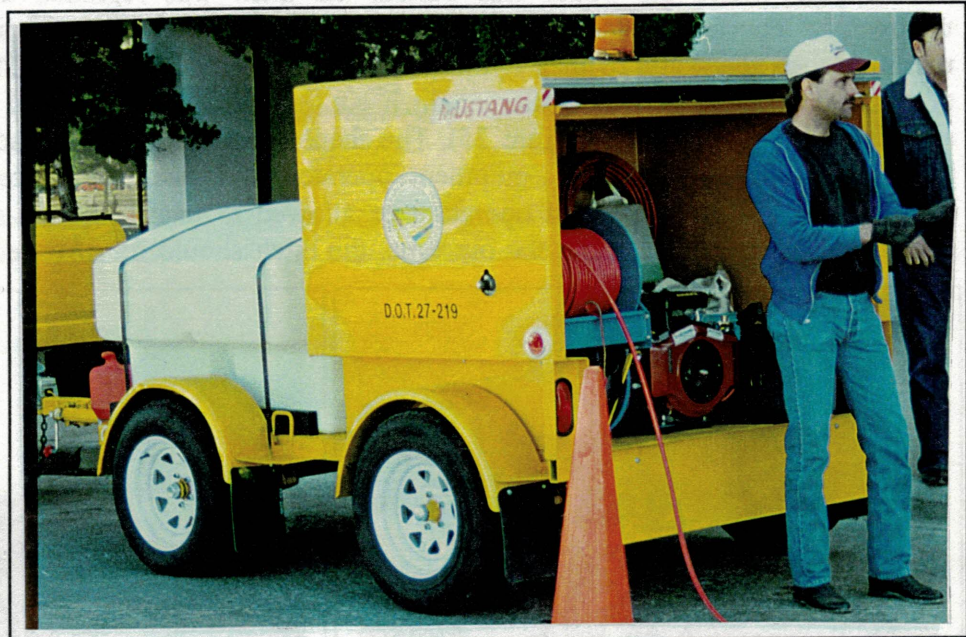
Figure 21 "Jetter" (High pressure rodding system.)
