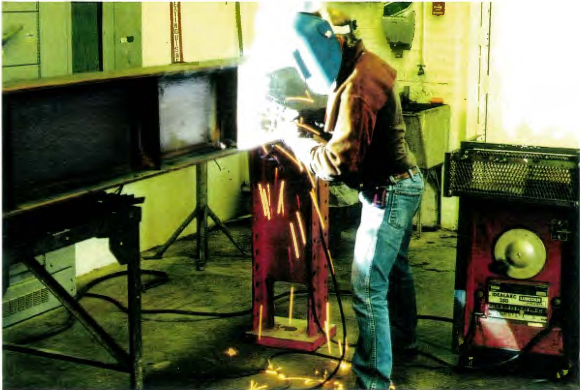
Figure 64. Welding a Test Specimen
