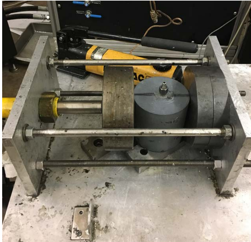
Figure 12: Uniaxial fracture test apparatus illustrating a single piston loading system on a cylindrical sample.
