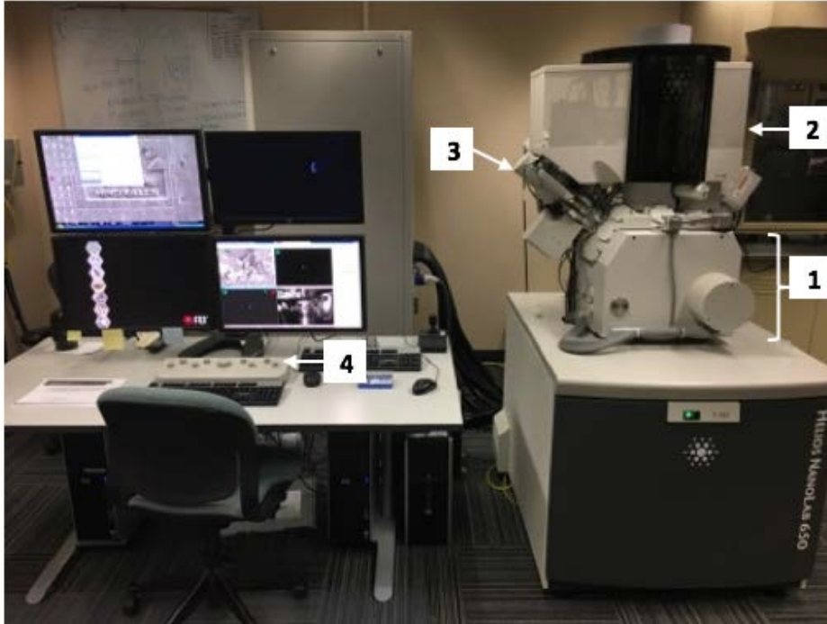
Figure 16: FEI HELIOS NANOLAB 650™ Scanning Electron Microscope with multicomputer software and analysis. (1) pressurized vacuum chamber; (2) electron column used to focus and illuminate the specimen; (3) electron gun produces the electron beam; (4) control panel.
