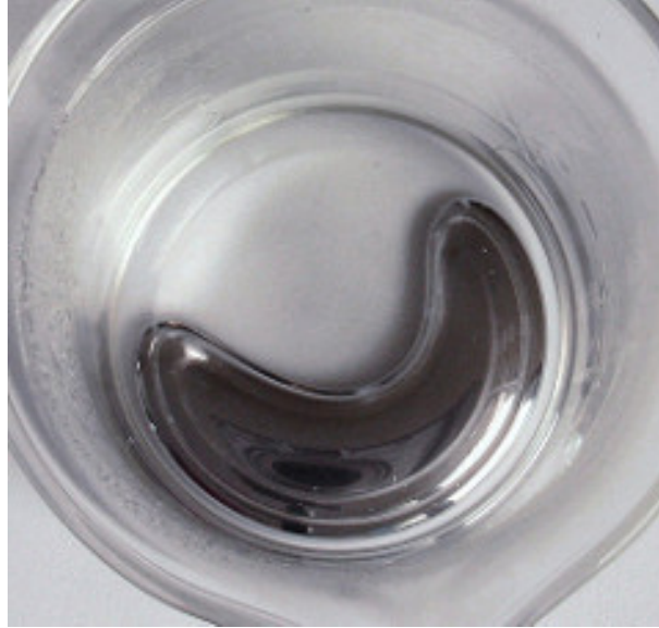
Figure 14: Liquid Field's metal at a temperature greater than 70°C. Field's metal is 32.5% Bismuth, 16.5% Tin, and 51% Indium (READE, 2018).
