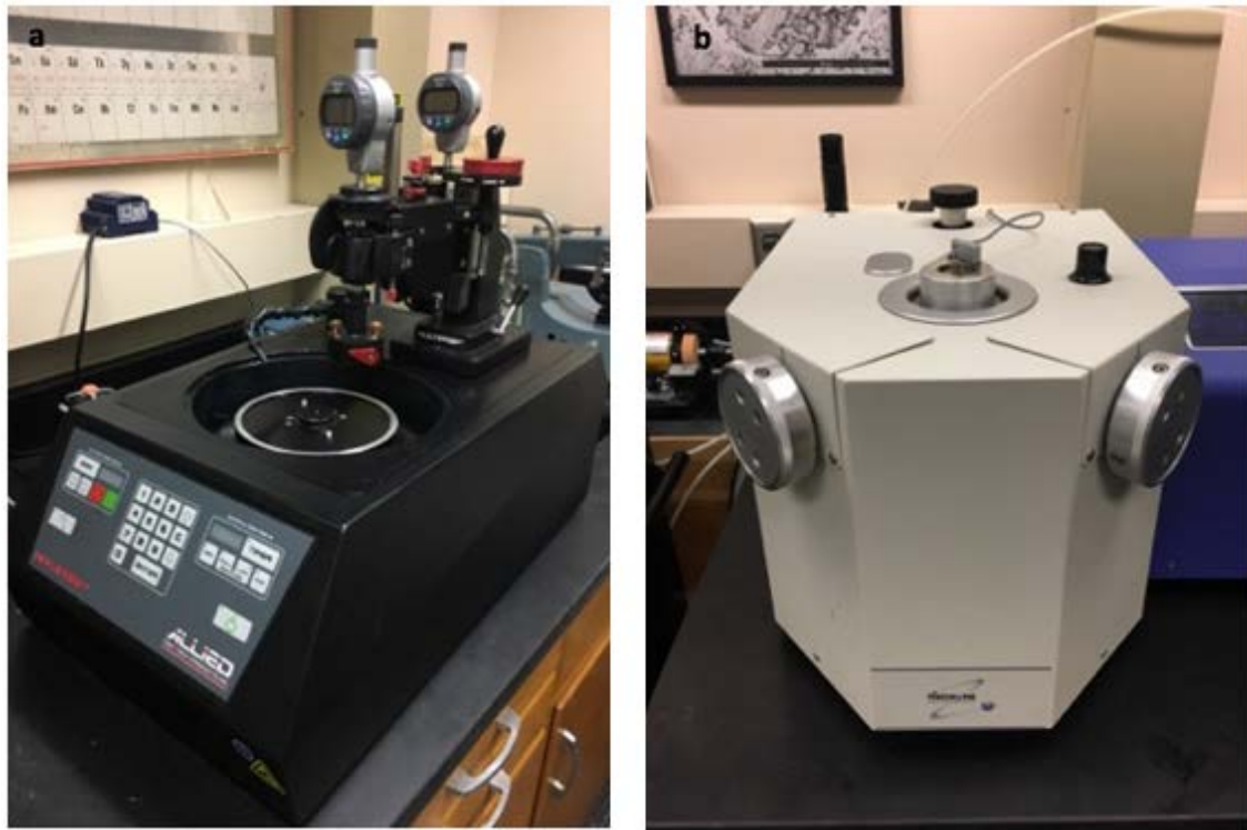
Figure 15: (a) Allied automatic polisher; (b) Model 1060™ Fischione ion mill. Allows molecular polishing on a 1-inch plug surface for superior SEM observation.
