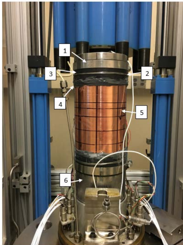
Figure 19: Core sample prepped for hydraulic fracture; (1) top metal spacer; (2) steel wire; (3) elastomeric tube; (4) epoxy between the rock sample, copper jacket, and elastomeric tube; (5) copper jacket; (6) bottom metal spacer.
