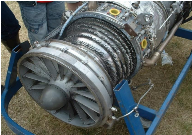
Fig. 1. 3 Damaged aircraft engine by a bird strike. (Wikipedia, 2009)
