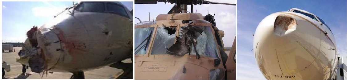
Fig. 1. 2 Damaged aircraft cockpit by bird strikes.
