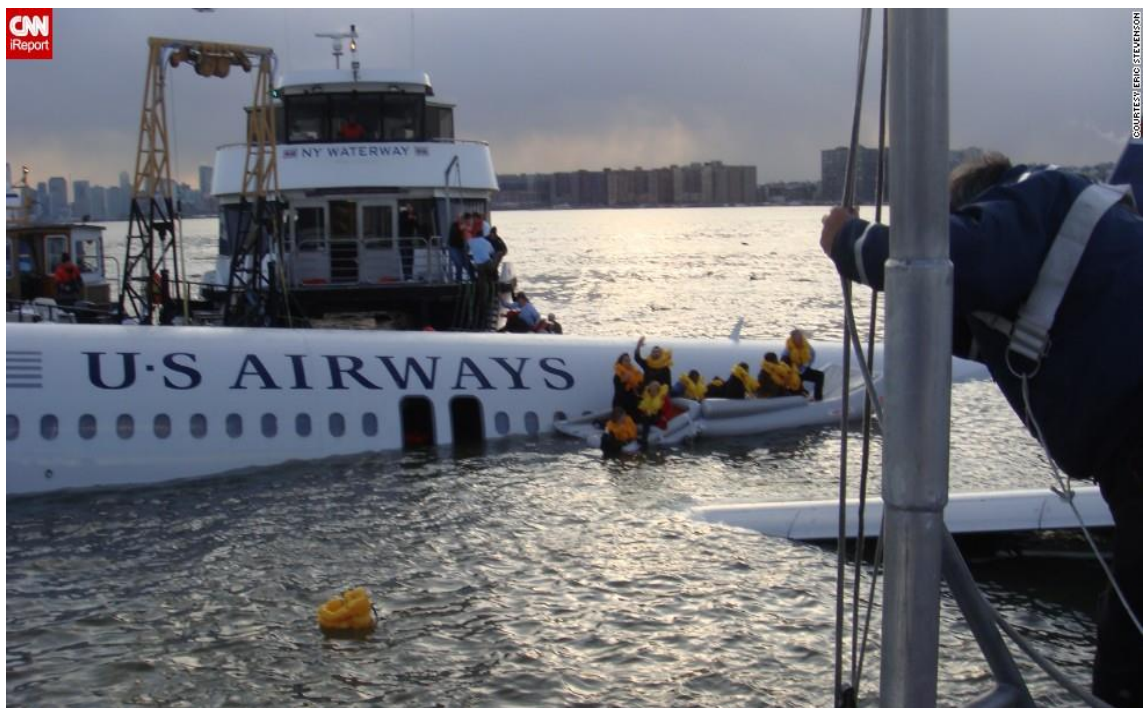
Fig. 1. 1 Hudson Landing of flight 1549 caused by engine shut down due to bird strike (Source: CNN)
