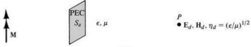
FIGURE 1.4: A PEC screen with a magnetic current source is analogous to the PMC screen in Figure 1.3.c [2].
