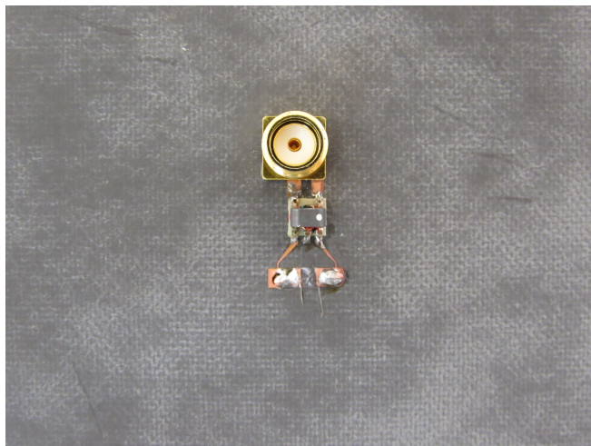
FIGURE 2.10: TC4-14+ connected to both sections of coupled microstrip on underside of the PIA.
