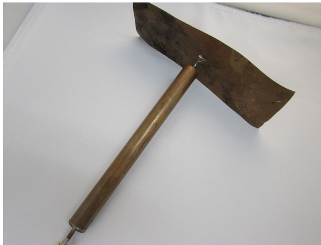
FIGURE 1.9: The balun shown in the figure is 6.75" in length, roughly the same length as the antenna's longest dimension.
