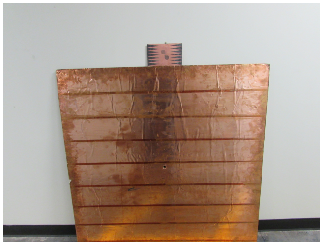
FIGURE 2.12: Ground plane (4' by 4') used to test PIA's placement insensitivity with new feeding techniques. The PIA is resting atop the ground plane to emphasize the size difference.
