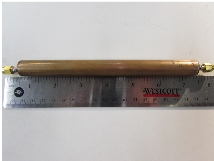
FIGURE 2.18: Sleeve balun designed for operation at 433 MHz; used in conjunction with PIA fed via chip balun.
