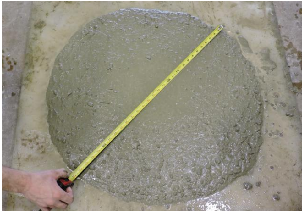
Figure D.4 Slump Flow Test Results of FR-SCC
