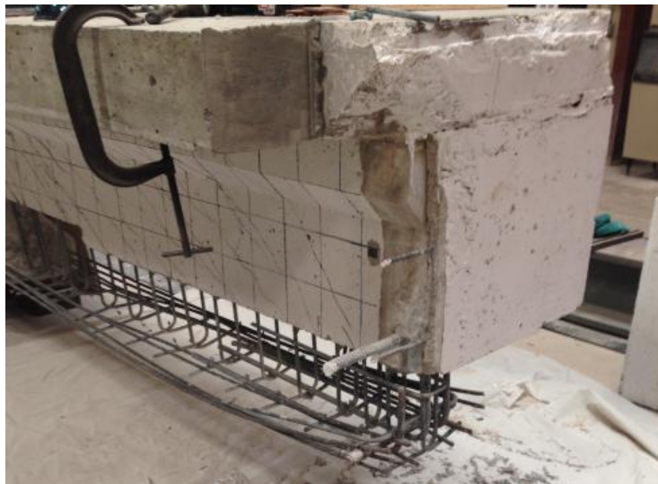
Figure 5.8 South End With Damaged Concrete Removed
