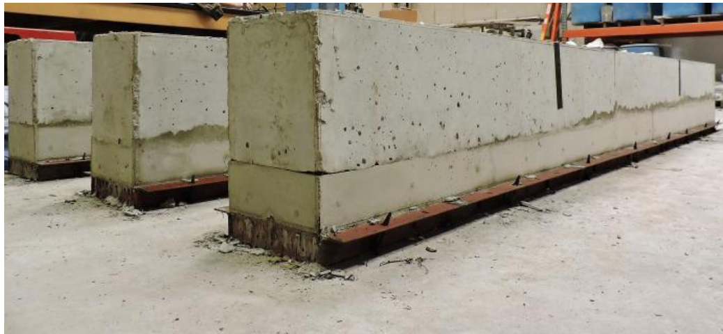
Figure 3.3 Three Finished FR-SCC Repair Beams (Wirkman, 2016)
