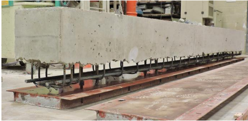
Figure 3.2 Repair Beam After Control Concrete & Before FR-SCC (Wirkman, 2016)
