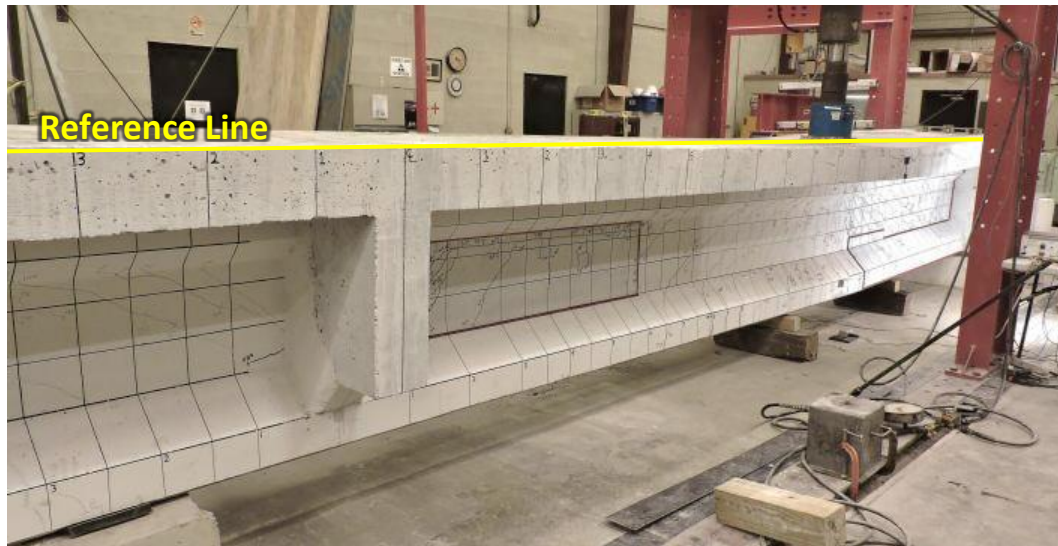
Figure 6.8 South End Test at Maximum Deflection
