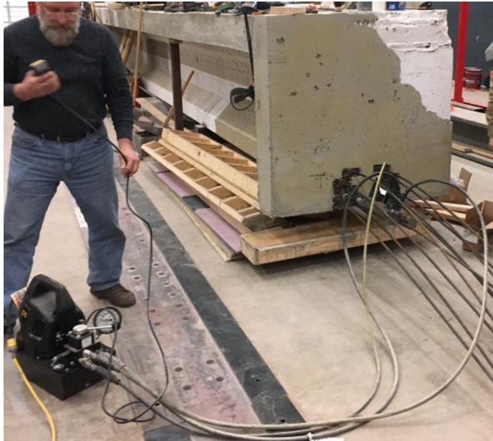
Figure 5.21 Post-Tensioning Strand Stressing
