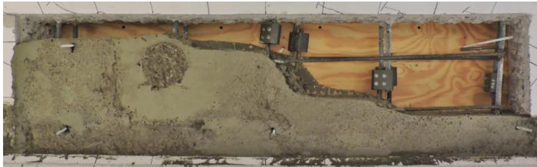
Figure 5.5 Extent of Flow for First Pour of Core-Sampled Web
