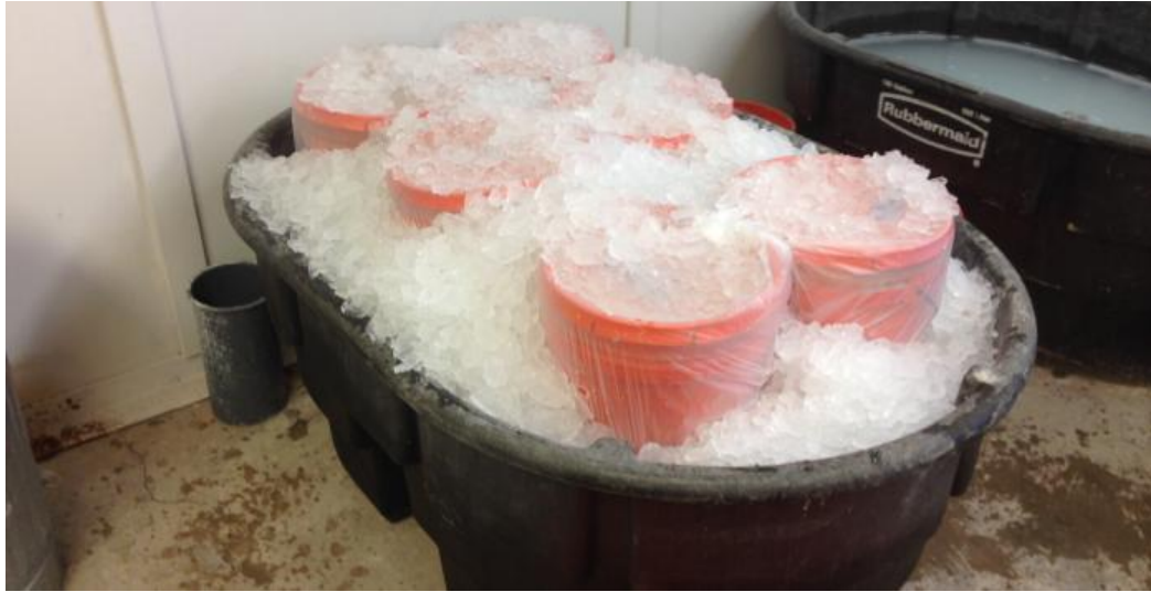
Figure 5.4 Mix Materials Chilled with Ice
