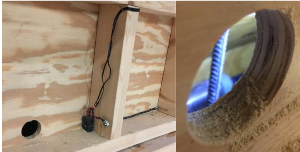
Figure 5.16 Observation Window for Monitoring Flow (Left) and View Through the Window (Right)
