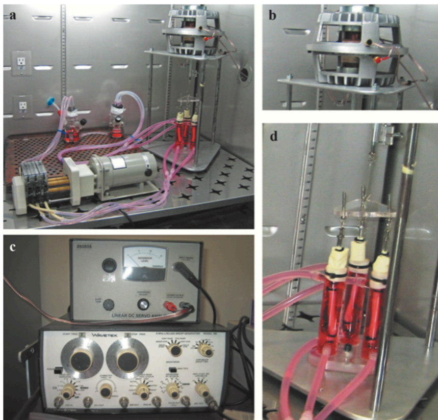
Figure 8. Bioreactor setup for tendon tissue engineering from OU research group[52].
