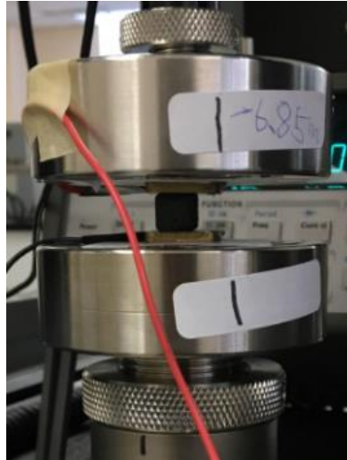
Figure 41. Electrical resistance measurement set up of porous nanocomposites created by the indirect method
