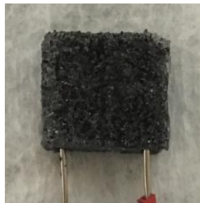
Figure 40. Electrical resistance measurement set up of porous nanocomposites created by the direct method
