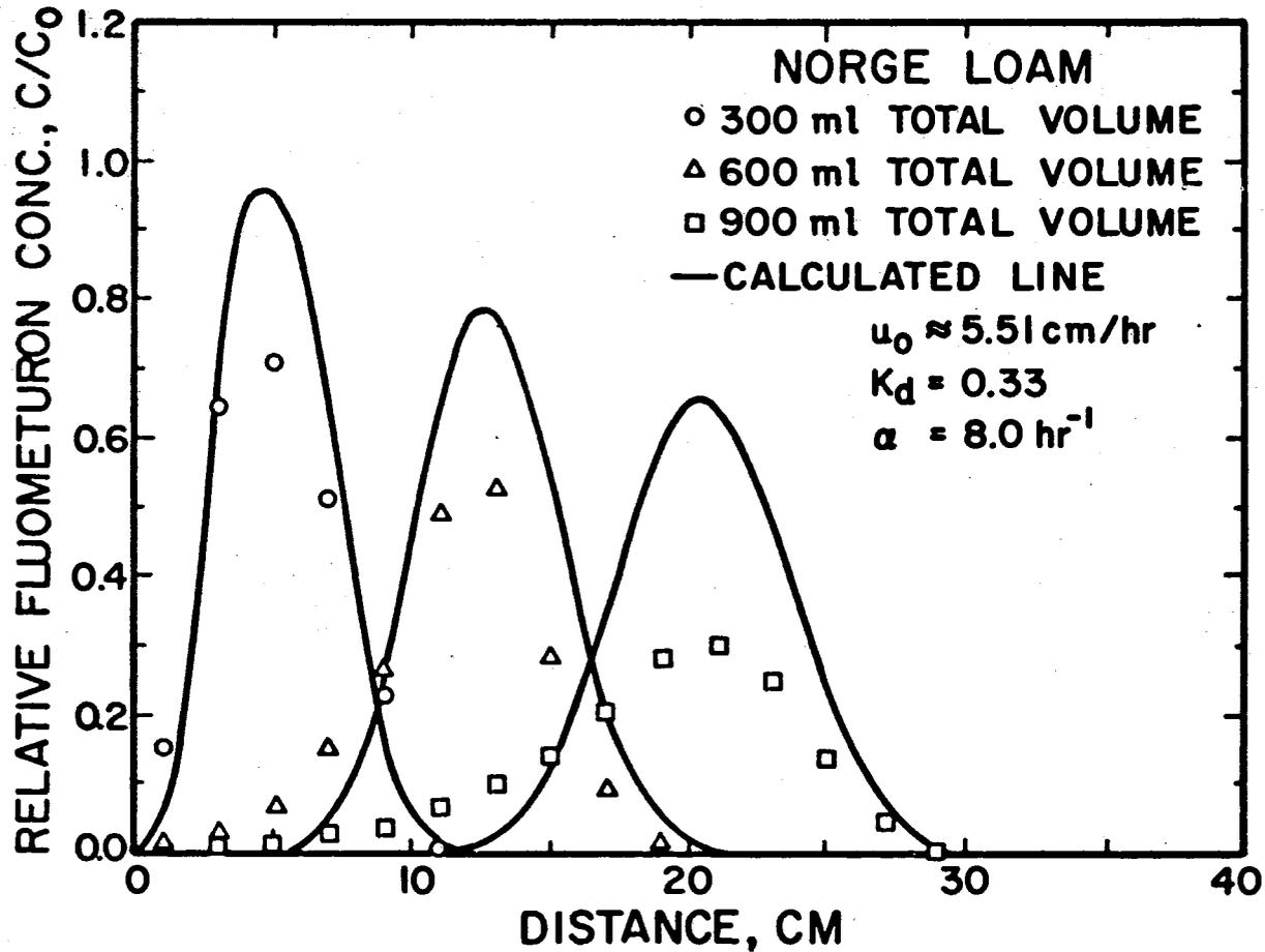
Figure 13. Experimental and Calculated Relative Fluometuron Solution Concentration Distributions in Norge Loam Soil Columns. Experimental Average Pore-Water Velocity Was 5.51 cm/hr. Solid Lines were Calculated Using Equation [17] (Oddson et al.) for  $u_0 = 5.51 \text{ cm/hr}$ ,  $K_d = 0.33 \text{ cm}^3/\text{hr}$ , and  $\alpha = 8.0 \text{ hr}^{-1}$ .
