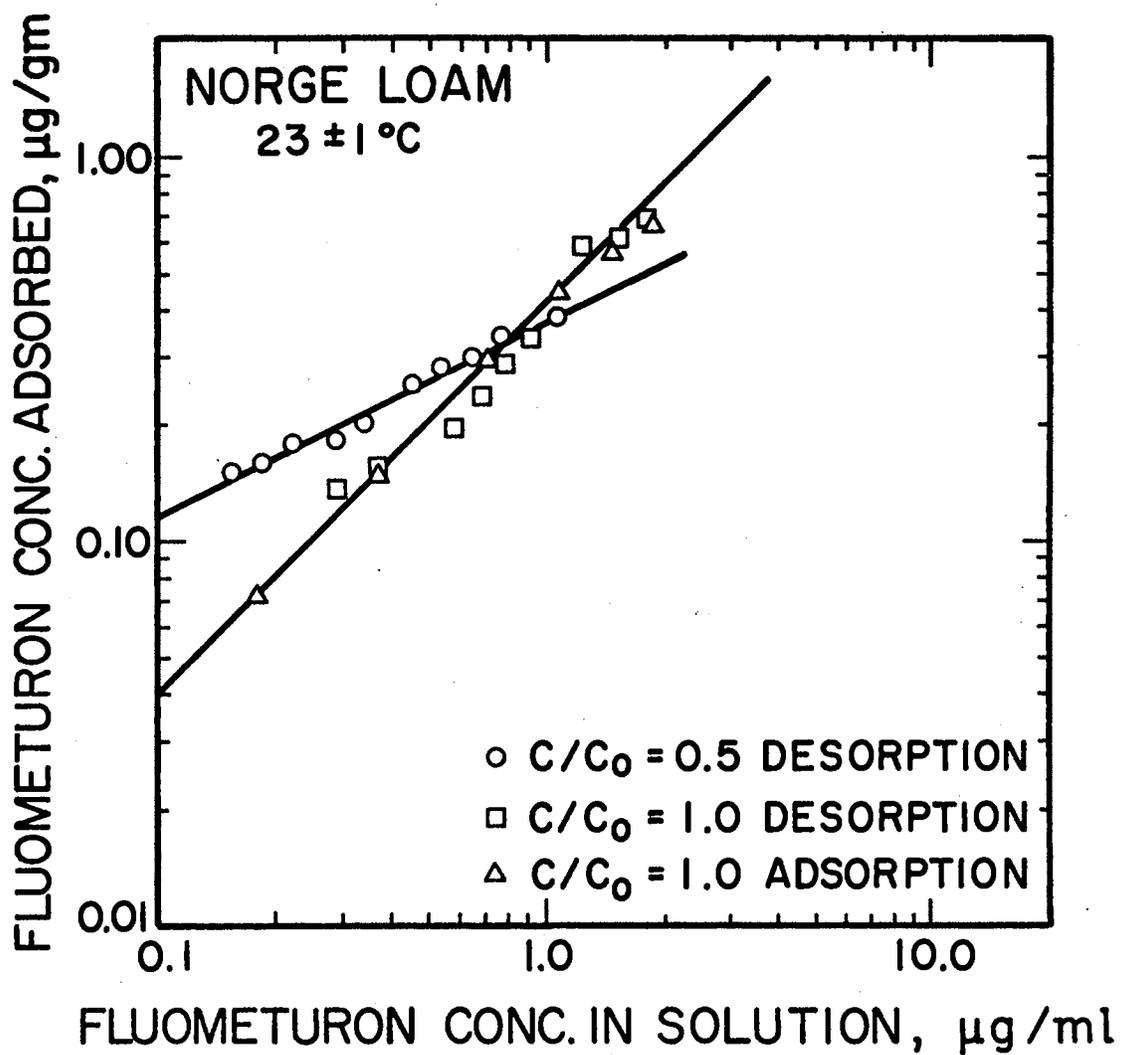
Figure 5. Desorption Isotherms for Fluometuron on Norge Loam Soil (5 gm Soil: 5 ml Fluometuron Solution) for 120 Minute Reaction Periods at Two Initial Adsorbed Fluometuron Concentrations. 120 Minute Adsorption Isotherm Given for Reference.
