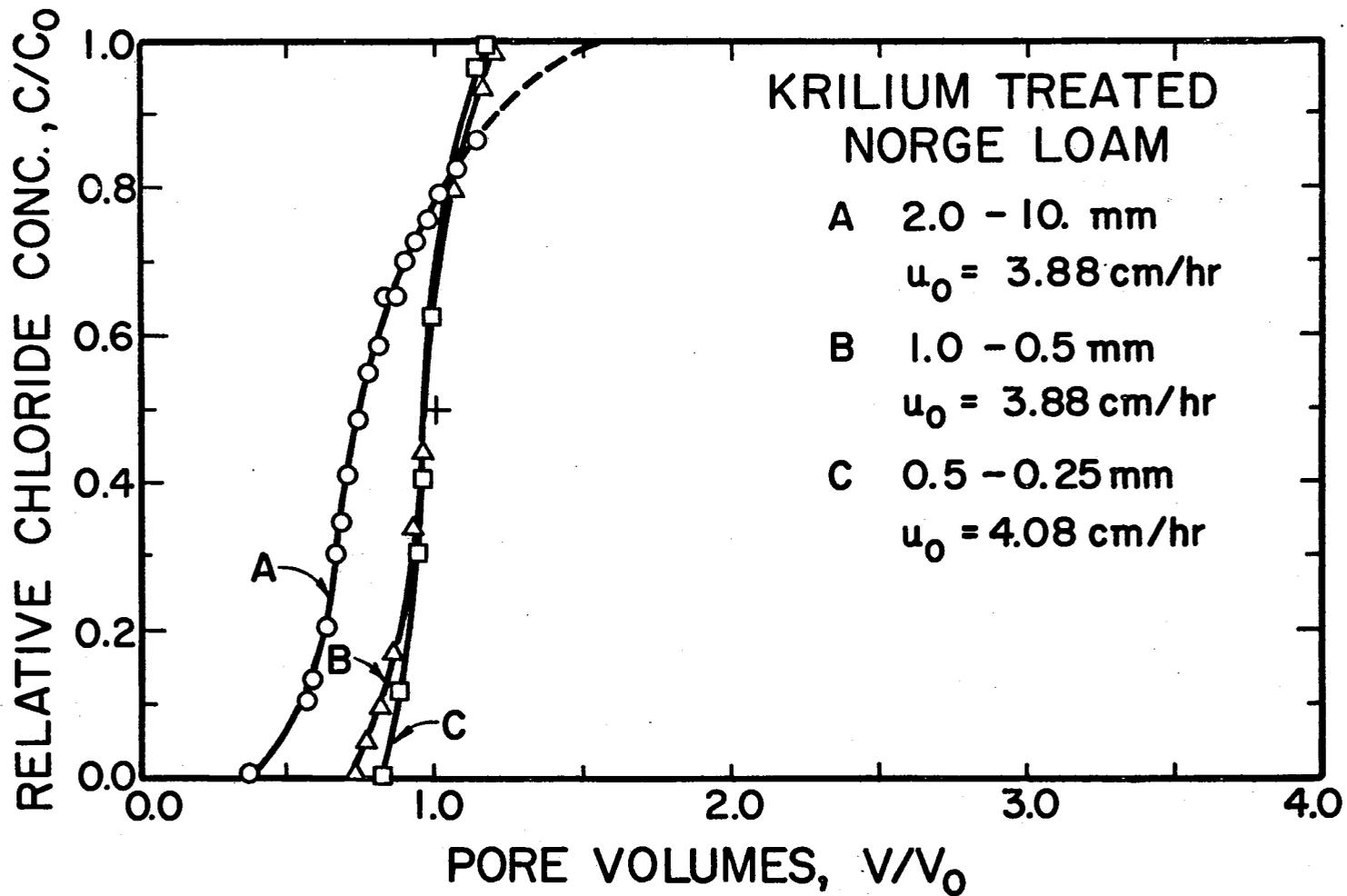
Figure 20. Relative Chloride Ion Concentration Distributions for 2.0 to 1.0, 1.0 to 0.5, and 0.5 to 0.25 mm Size Stabilized Aggregates at 3.88, 3.88, and 4.08 cm/hr Average Pore-Water Velocities Respectively.
