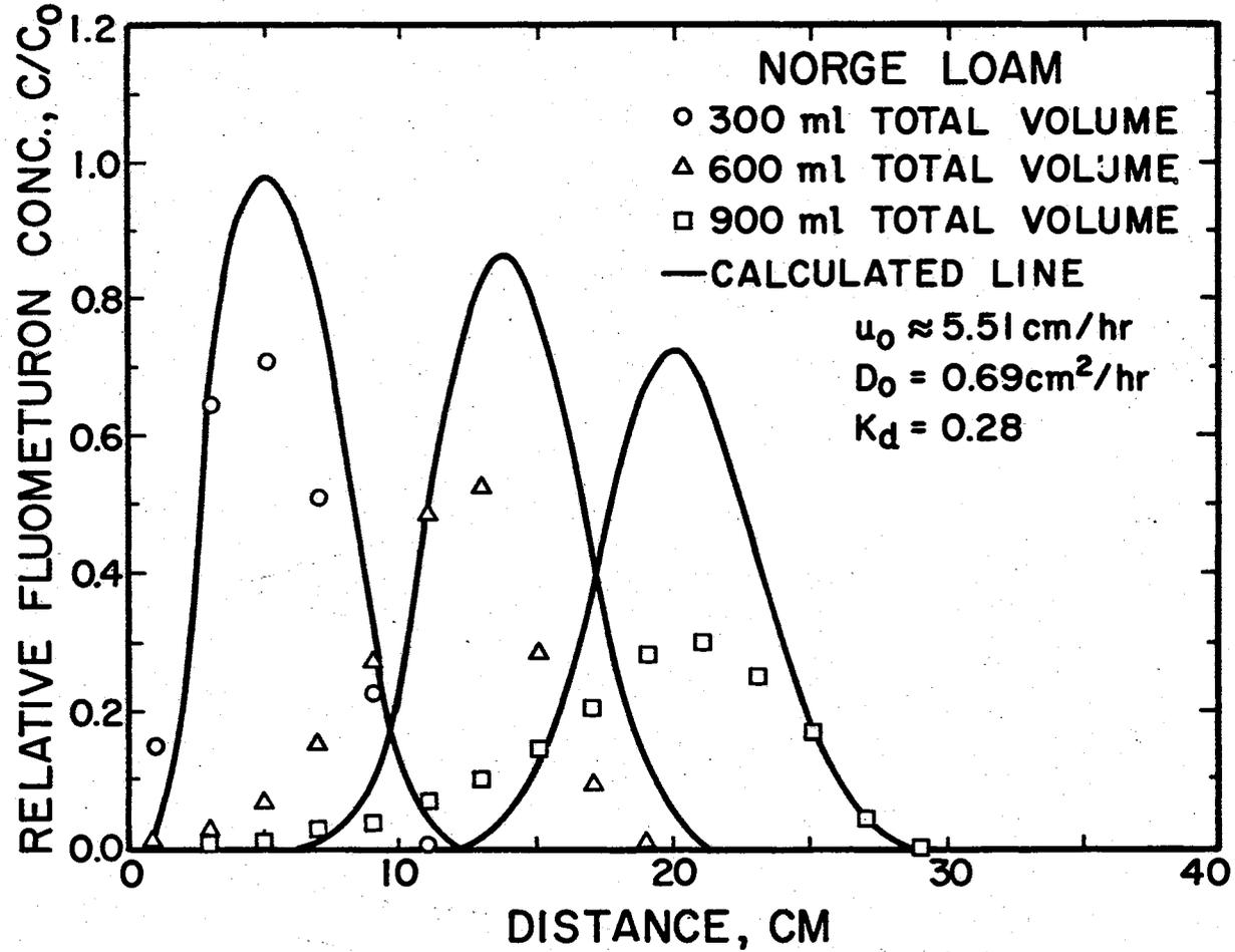
Figure 10. Experimental and Calculated Relative Fluometuron Solution Concentration Distributions in Norge Loam Soil Columns. Experimental Average Pore-Water Velocity Was 5.51 cm/hr. Solid Lines Were Calculated Using Equation [6] (Davidson et al.) for  $u_0 = 5.51 \text{ cm/hr}$ ,  $D_0 = .069 \text{ cm}^2/\text{hr}$ , and  $K_d = 0.28 \text{ cm}^3/\text{gm}$ .
