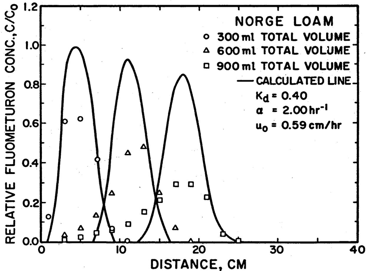
Figure 12. Experimental and Calculated Relative Fluometuron Solution Concentration Distributions in Norge Loam Soil Columns. Experimental Average Pore-Water Velocity Was 0.59 cm/hr. Solid Lines Were Calculated Using Equation [17] (Oddson et al.) for  $u_0 = 0.59 \text{ cm/hr}$ ,  $K_d = 0.40 \text{ cm}^3/\text{hr}$ , and  $\alpha = 2.0 \text{ hr}^{-1}$ .
