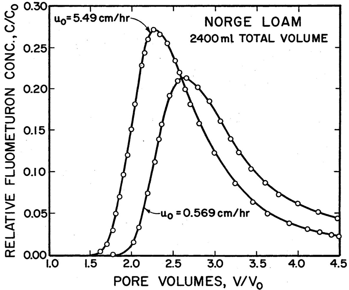
Figure 16. Relative Fluometuron Effluent Solution Concentration Distribution Curves for 2400 ml Total Throughput Volumes at Average Pore-Water Velocities of 5.49 cm/hr and 0.569 cm/hr.
