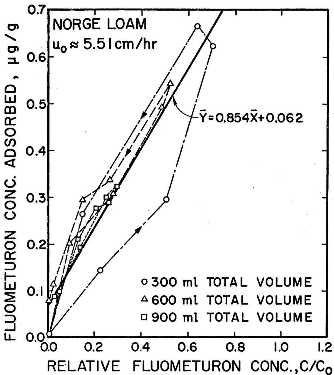
Figure 6. Transient Adsorption-Desorption Behavior of Fluometuron in Norge Loam Soil Columns With an Average Pore-Water Velocity of 5.51 cm/hr.
