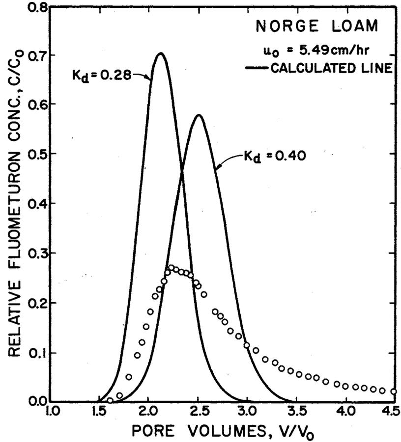
Figure 17. Experimental and Calculated Relative Fluometuron Effluent Solution Concentration Distributions for 2400 ml Total Throughput Volume at an Average Pore-Water Velocity of 5.49 cm/hr. Solid Lines Calculated Using Equation [6] (Davidson et al.) with  $D_0 = 0.69 \text{ cm}^2/\text{hr}$  and  $K_d = 0.28 \text{ cm}^3/\text{hr}$ , and  $D_0 = 0.69 \text{ cm}^2/\text{hr}$ , and  $K_d = 0.40 \text{ cm}^3/\text{hr}$ .
