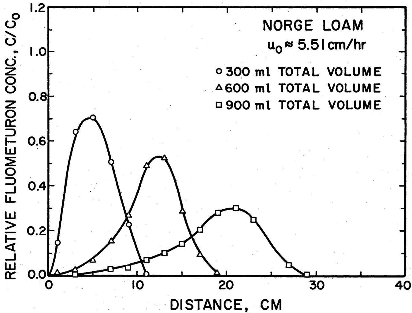
Figure 8. Relative Fluometuron Solution Concentration Distributions in Norge Loam Soil Columns for an Average Pore-Water Velocity of 5.51 cm/hr.
