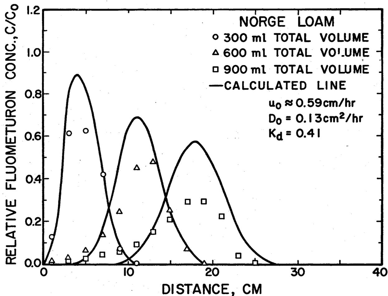
Figure 11. Experimental and Calculated Relative Fluometuron Solution Concentration Distributions in Norge Loam Soil Columns. Experimental Average Pore-Water Velocity Was 0.59 cm/hr. Solid Lines Were Calculated Using Equation [6] (Davidson et al.) for  $u_0 = 0.59 \text{ cm/hr}$ ,  $D_0 = 0.13 \text{ cm}^2/\text{hr}$ , and  $K_d = 0.41 \text{ cm}^3/\text{gm}$ .
