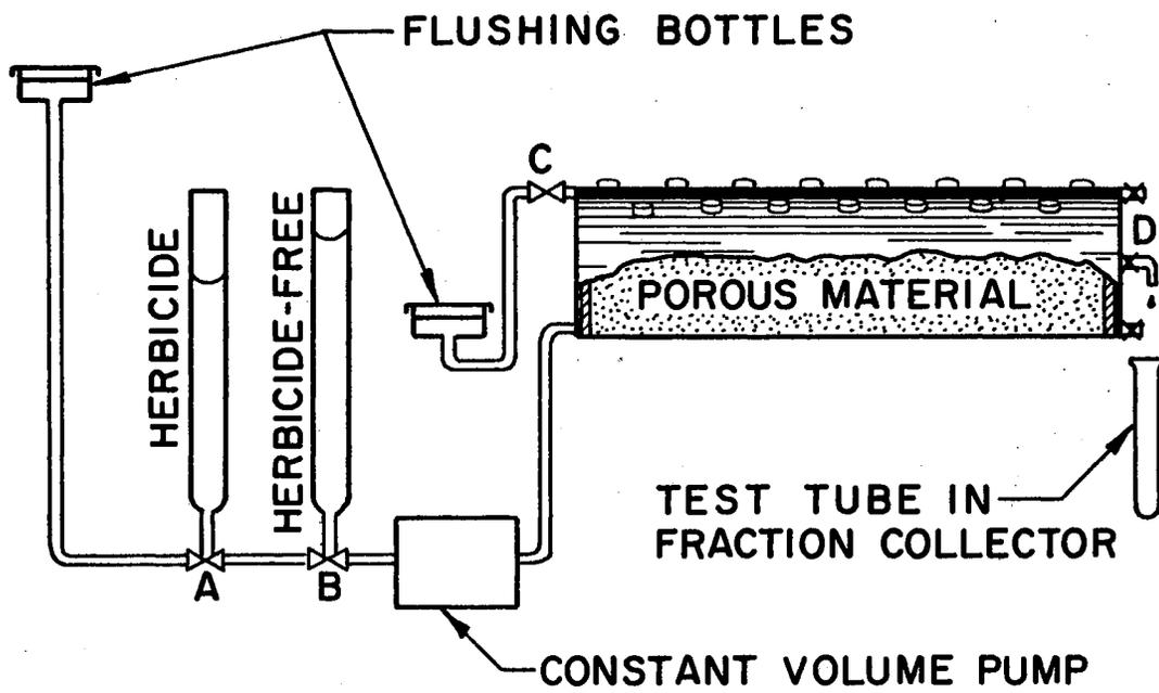
Figure 2. Apparatus Used in Miscible Displacement Study
