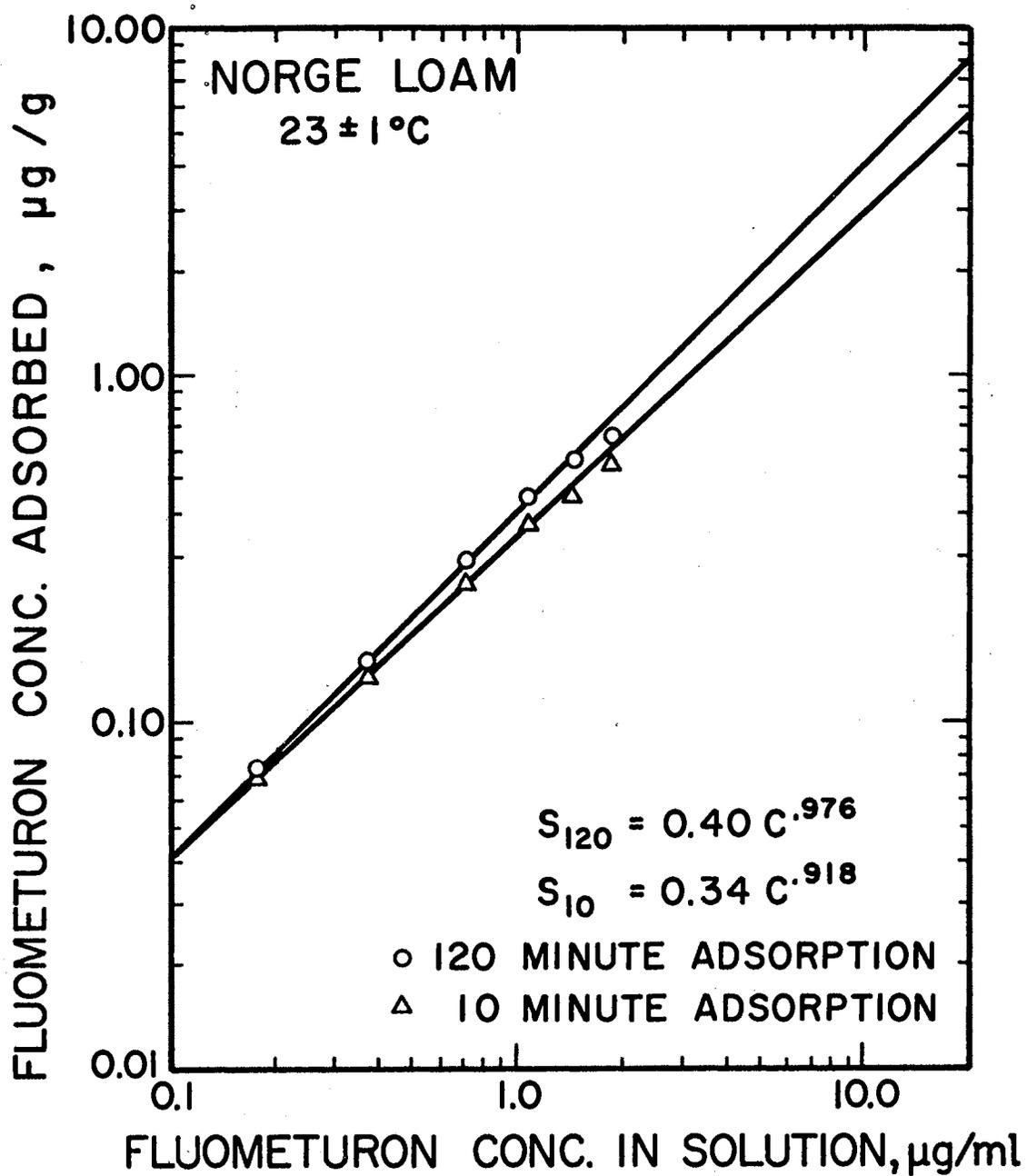
Figure 4. Adsorption Isotherms for Fluometuron on Norge Loam Soil (5 gm Soil: 5 ml Fluometuron Solution) Following 10 and 120 Minute Reaction Period
