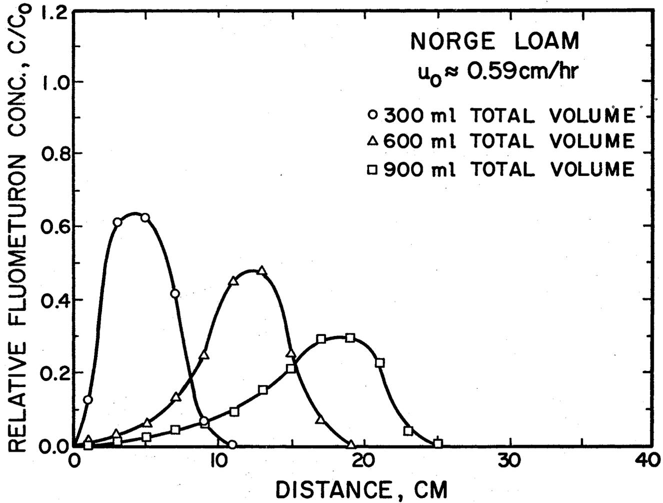
Figure 9. Relative Fluometuron Solution Concentration Distributions in Norge Loam Soil Columns for an Average Pore-Water Velocity of 0.59 cm/hr.
