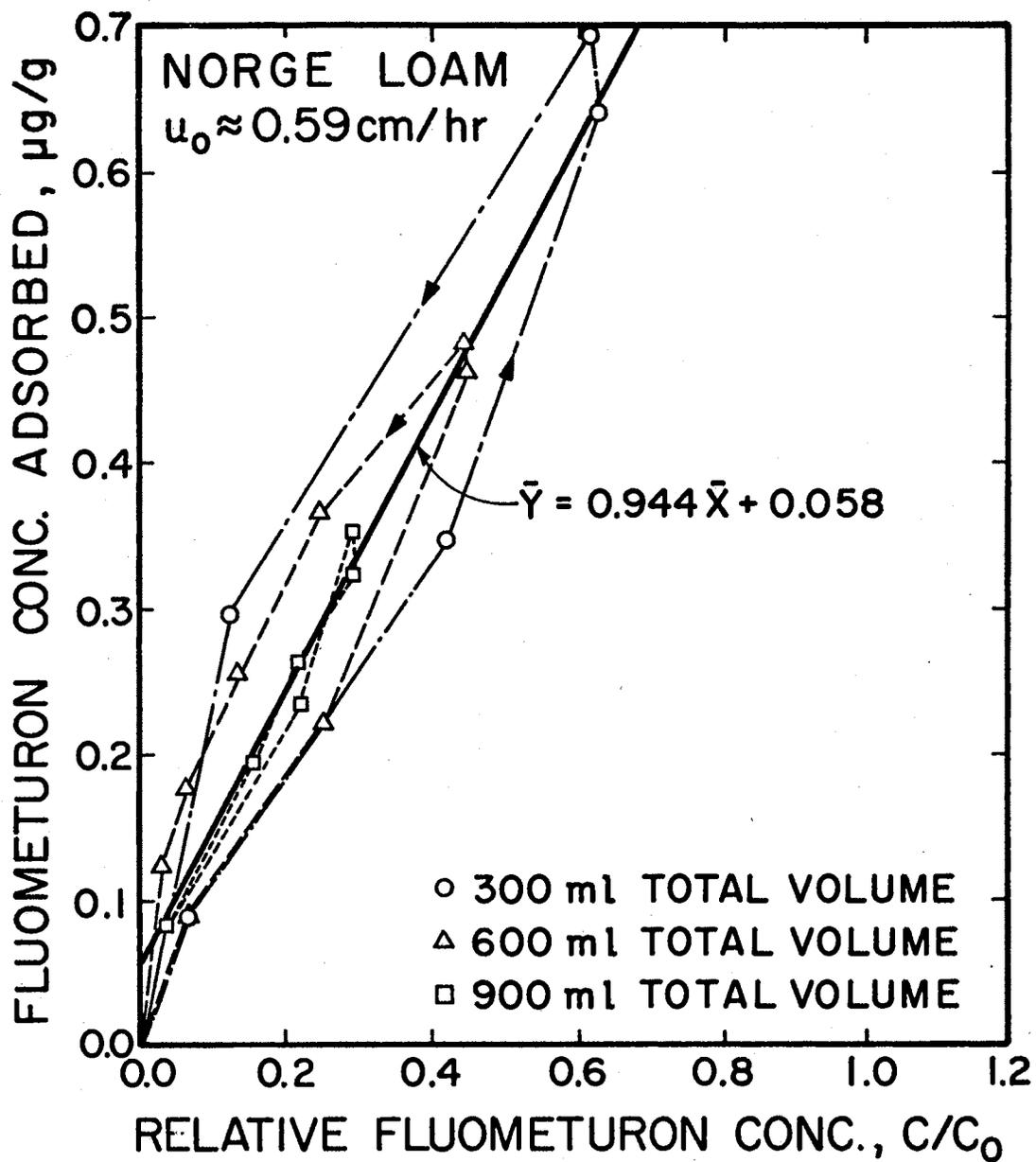
Figure 7. Transient Adsorption-Desorption Behavior of Fluometuron in Norge Loam Soil Columns With an Average Pore-Water Velocity of 0.59 cm/hr.
