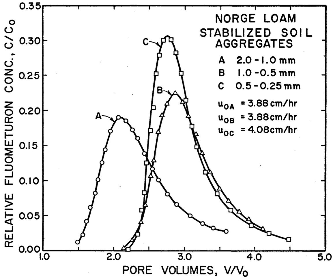
Figure 19. Relative Fluometuron Effluent Solution Concentration Distributions for 2.0 to 1.0, 1.0 to 0.5, and 0.5 to 0.25 mm Size Stabilized Aggregates at 3.88, 3.88, and 4.08 cm/hr Average Pore-Water Velocities Respectively.
