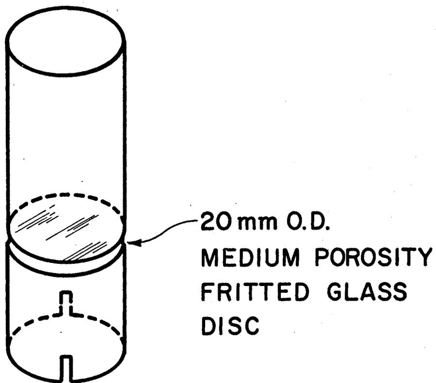
Figure 3. Apparatus Used To Separate Adsorbed and Nonadsorbed Fluometuron Phases
