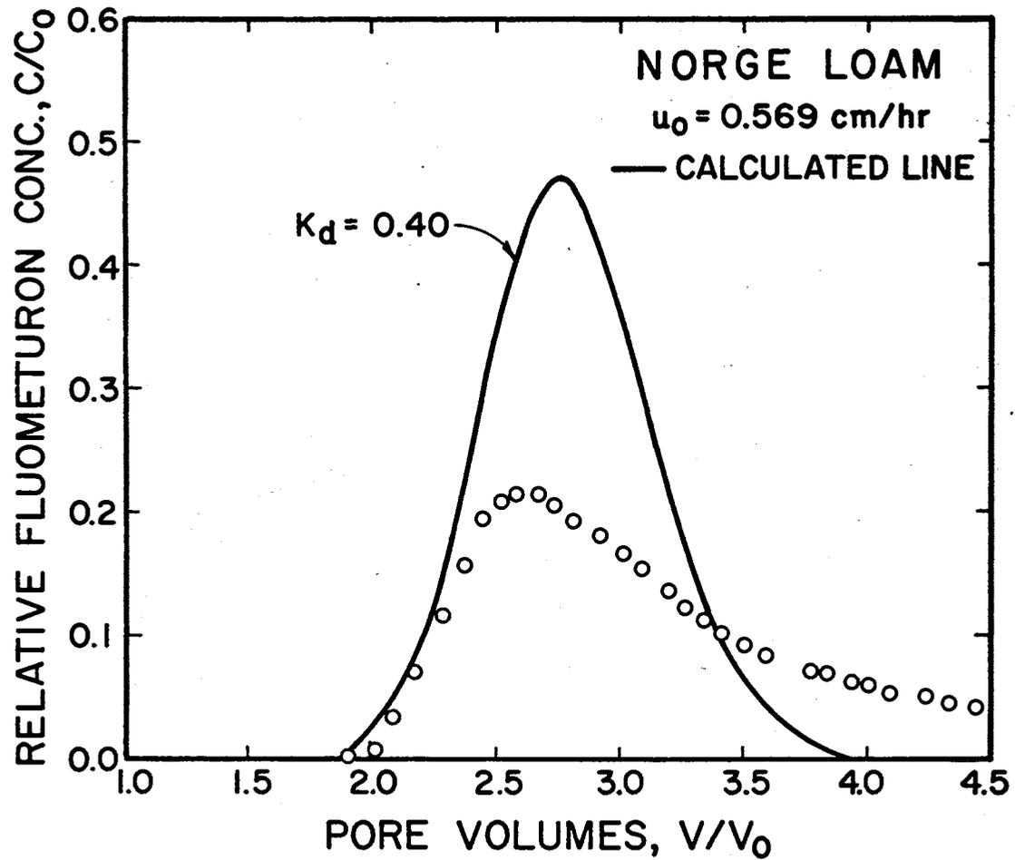
Figure 18. Experimental and Calculated Relative Fluometuron Effluent Solution Concentration Distributions for 2400 ml Total Throughput Volume at an Average Pore-Water Velocity of 0.569 cm/hr. Solid Lines Calculated Using Equation [6] (Davidson et al.) With  $D_0 = 0.13 \text{ cm}^2/\text{hr}$  and  $K_d = 0.40 \text{ cm}^3/\text{hr}$ .
