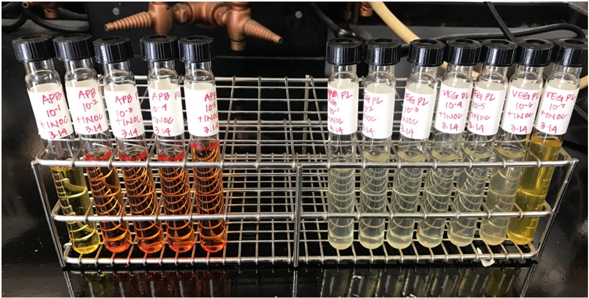
Figure 4. APB media comparisons. On the left is the standard phenol red medium and on the right, is the RST-APB medium. Red indicates no growth. Yellow or clear indicates growth.
