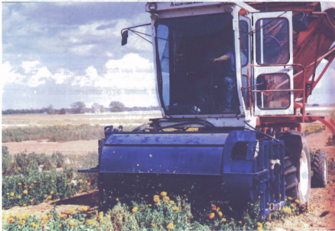
Figure 4. Retractable Finger Header on Allis Cotton Stripper.
