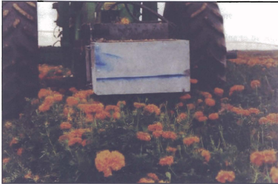
Figure 10. Fixed finger header mounted on John Deere tractor.
