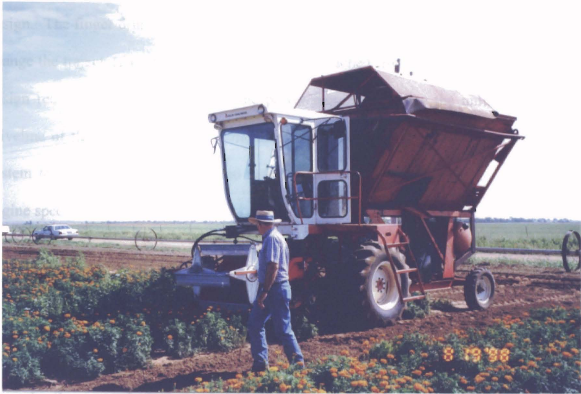
Figure 5. Direct cut header on Allis Chalmers cotton stripper.
