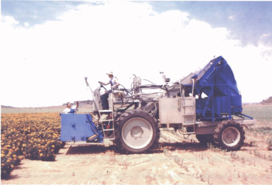
Figure 11. Fixed finger header on Chisholm Ryder harvester.
