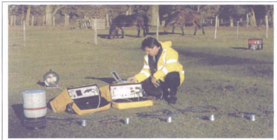
Figure 3. A field computer running a seismic test ( www.gdsinstruments.com )
