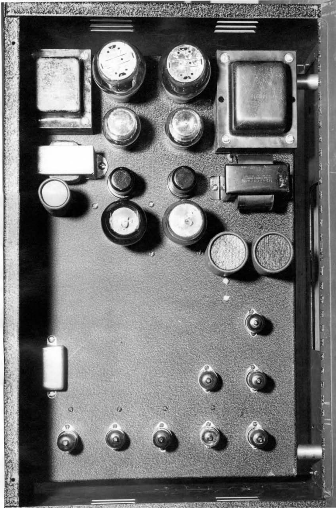
Figure 11 Top View of Trigger Circuit and Power Supply Chassis.
