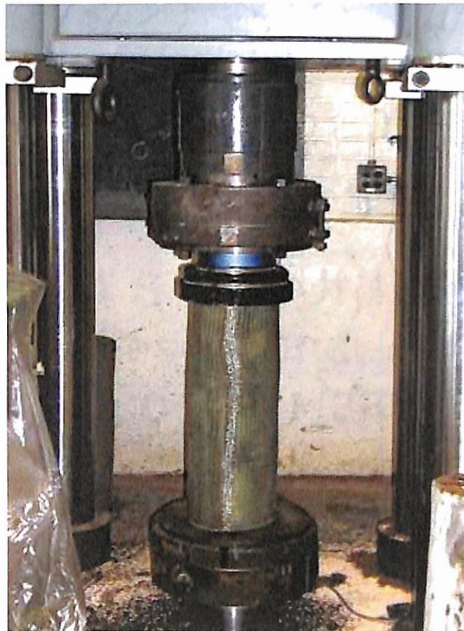
FIG. 4.2. Typical Setup for Compression Testing of Laboratory Repaired Timber Piles
