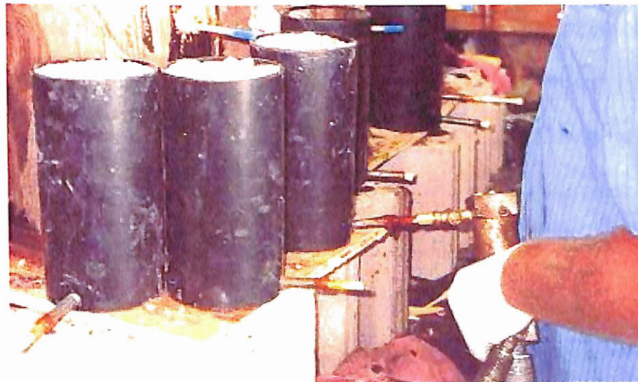
FIG. 3.1. Injection of Low Viscosity Epoxy Resin
