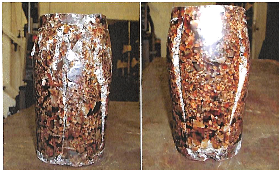
FIG. 5.2. Compression Failure of Unreinforced Laboratory Fabricated Cylinders
