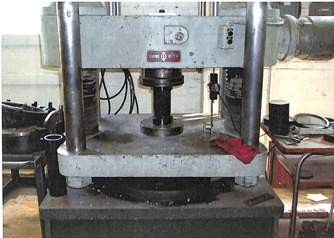
FIG. 4.1. Typical Setup for Compression Testing of Laboratory Fabricated Cylinders
