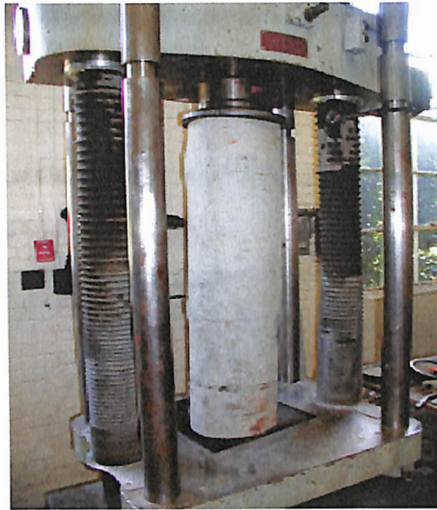
FIG. 3.3. Field Repaired Timber Pile
