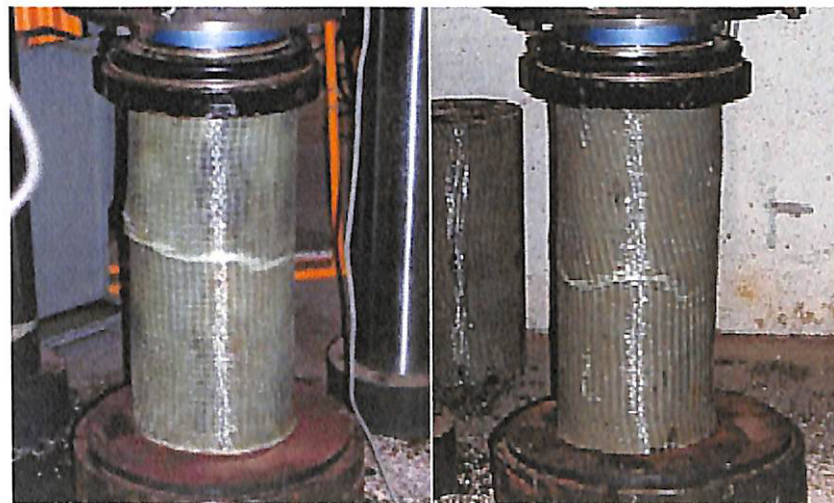
FIG. 5.12. Compression Failure of Core-repaired Timber Piles with Transverse Reinforcement
