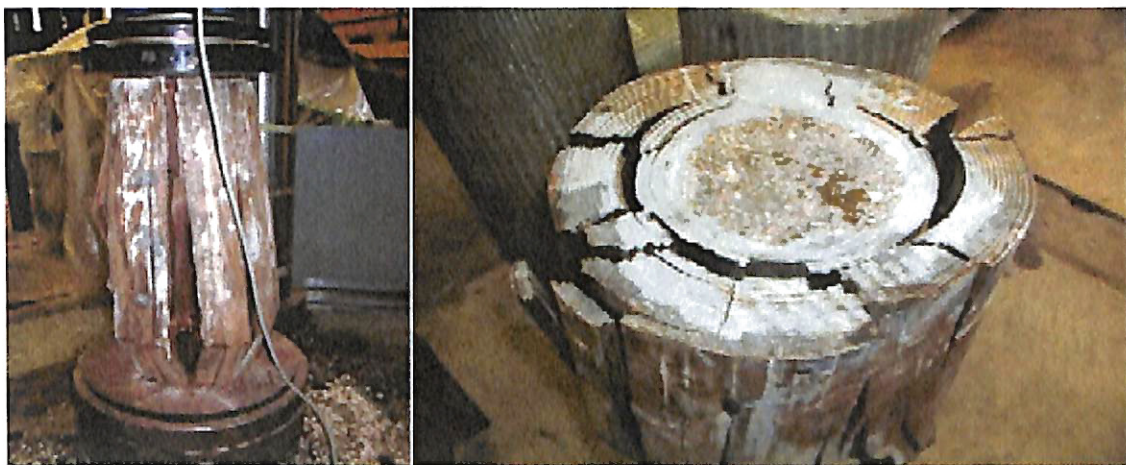
FIG. 5.10. Compression Failure of Core-repaired Timber Piles
