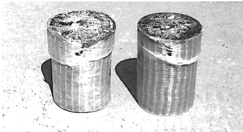
FIG. 5.6. Compression Failure of Laboratory Fabricated Cylinders with Transverse and Longitudinal Fiberglass Reinforcement
