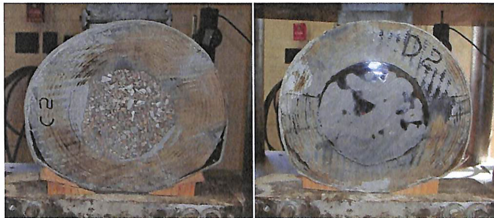
FIG. 5.23. Delamination of Fiberglass Reinforcement
