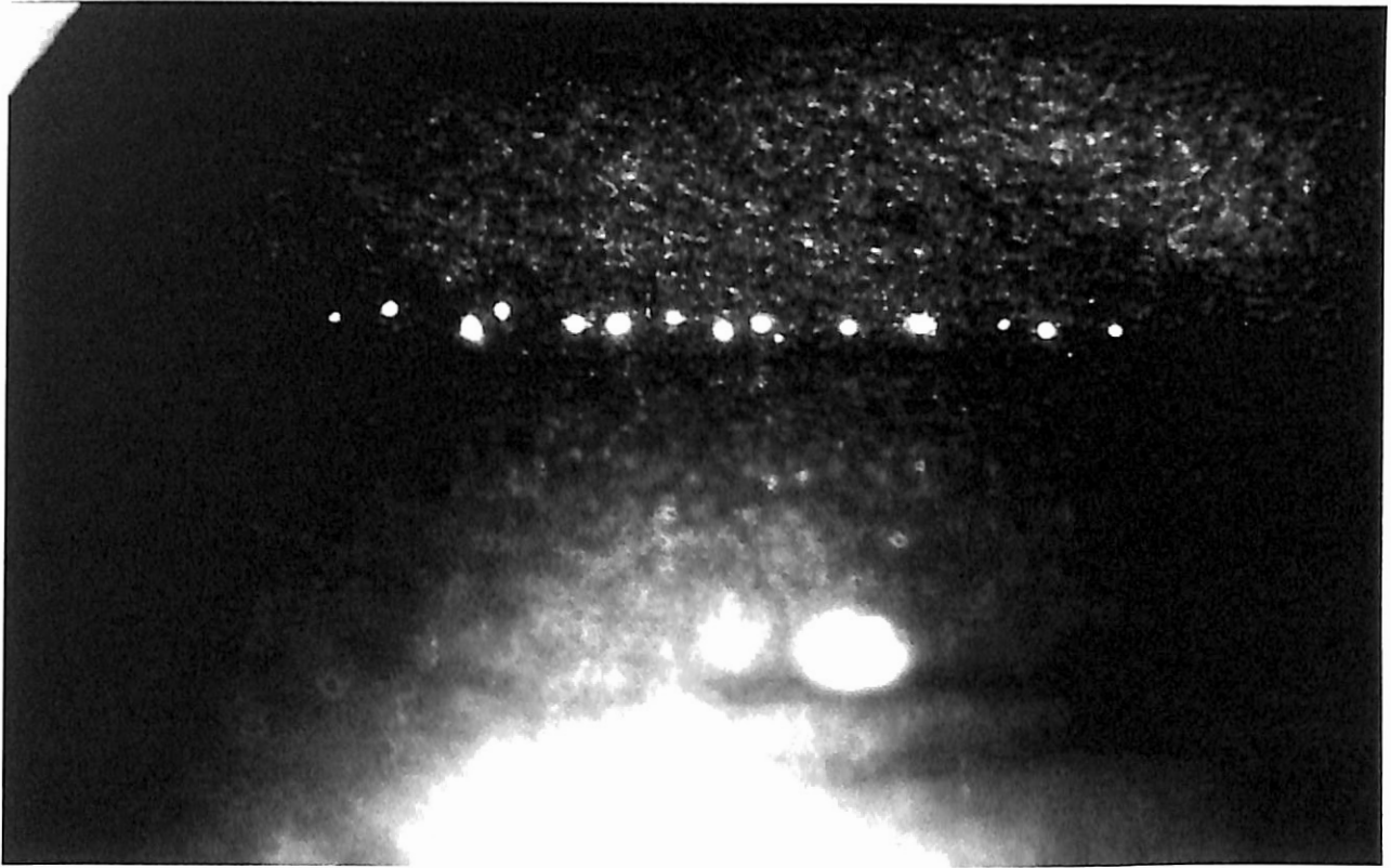
Figure 16: Nano-particle core fluorescence (OG-590 filter), 0.04 second exposure time, beads not exposed to analyte. Picture made from 4 meter distance using f/1.8 lens
