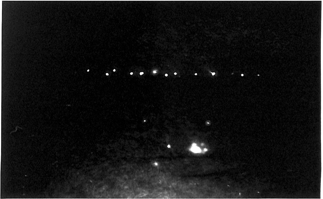
Figure 15: AFP fluorescence (blue filter), 2 second exposure time, beads not exposed to analyte. Picture made from 4 meter distance using f/1.8 lens
