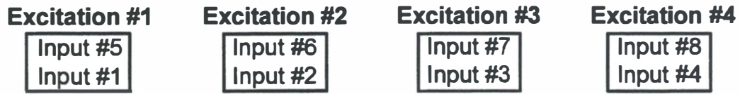
Figure 10. Excitation Arrays. Each excitation channel services two Input channels to make up an Excitation Array.
