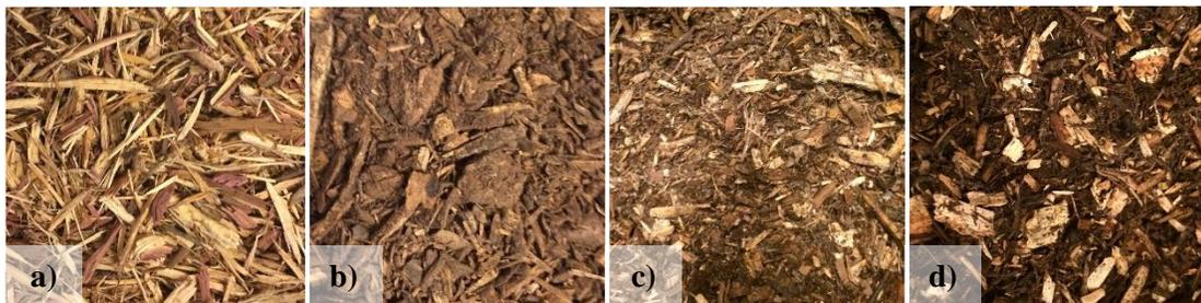
**Figure 3.3:** Image of the mulch used in single material testing. From left to right: a) shredded, b) high degradation chipped, c) medium degradation chipped, and d) low degradation chipped eastern red cedar mulch.
