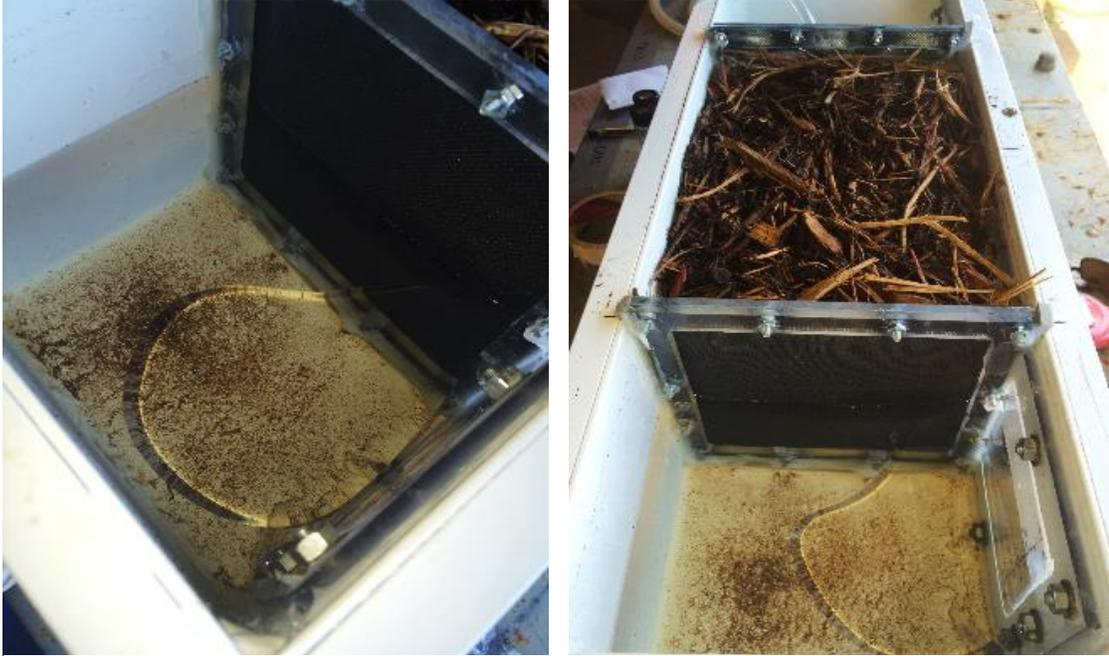
**Figure 3.2:** Images of fuel breakthrough into the bio-separator's fuel storage reservoir. Bio-separator tests were concluded at time of breakthrough. Both images are of shredded mulch replicate B test.
