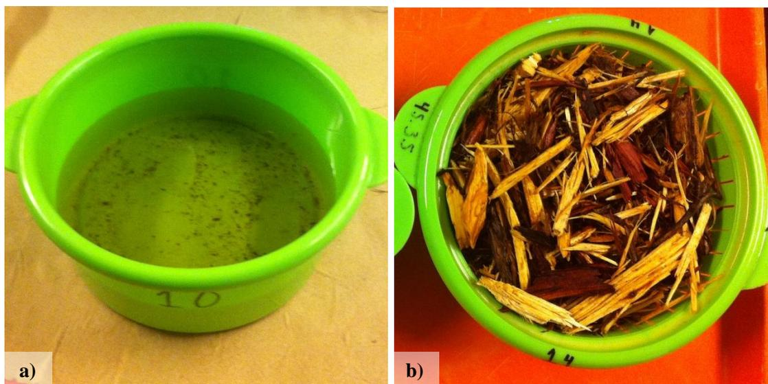
**Figure 3.9:** Example images of mulch liquid-uptake experiments. a) shows the vegetable steamer reservoir with water and loose soil after an experiment and b) shows the strainer compartment filled with medium-degraded shredded mulch during an experiment.
