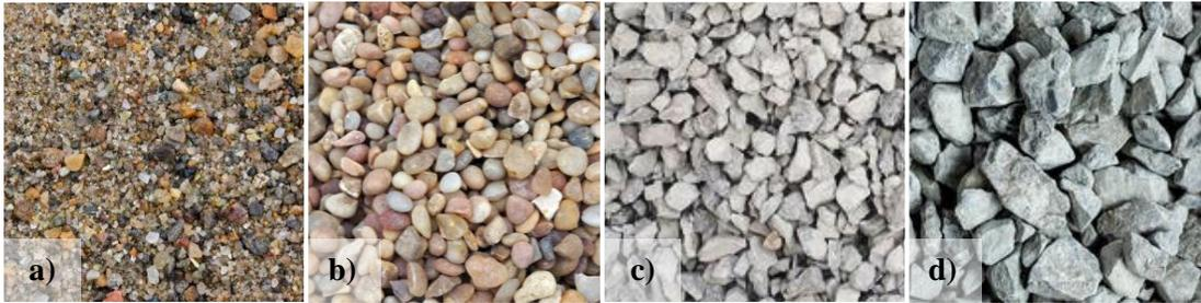
**Figure 3.4:** Image of the aggregate materials used for single material testing. From left to right: a) concrete sand, b) pea gravel, c) small crushed limestone (size #8), and d) large crushed limestone (size #4).
