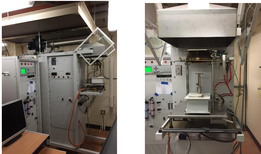
Fig. 5 Experimental Set-up for Cone Calorimeter.
