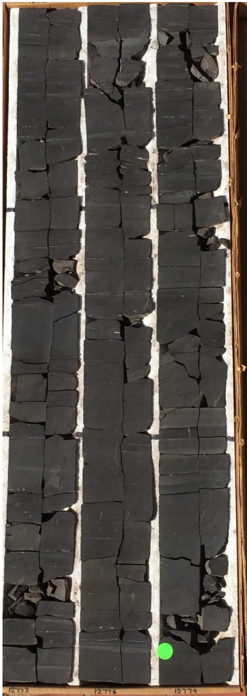
Appendix A. Williams 1H-7X core photographs of subsea depths 12,779 feet to 12,770 feet (middle figure). Depth shallows from bottom right corner to top left corner at a thickness of 3 feet per column in core box.
