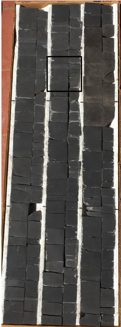
Appendix B. McDonald 2H-16E core photographs of subsea depths 6,373 feet to 6,364 feet (left figure). Depth shallows from bottom right corner to top left corner at a thickness of 3 feet per column in core box. Evident inverse grading in silica-rich laminae and pyrite laminae occur from 6,364.6 to 6,364.4 feet (upper right).
