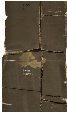
Appendix B. McDonald 2H-16E core photographs of subsea depths 6,381.9 feet to 6,373 feet (far left figure). Depth shallows from bottom right corner to top left corner at a thickness of 3 feet per column in core box. Pyrite burrows occur from 6,374.1 feet to 6,373.9 feet (left figure). PPL and XPL of silt to sand-sized possible radiolarians displaying undulatory chalcedony at 6,380.35 feet (bottom right).
