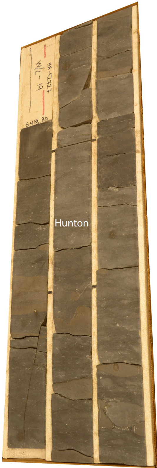
Appendix B. McDonald 2H-16E core photographs of subsea depths 6,427 feet to 6,418 feet (left figure). Depth shallows from bottom right corner to top left corner at a thickness of 3 feet per column in core box. Varying macrofossils such as ostracods and brachiopods occur at 6,428.55 feet, PPL (upper right).
