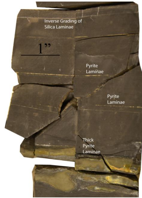
Appendix A. Williams 1H-7X core photographs of subsea depths 12,869 feet to 12,860 feet (left figure). Depth shallows from bottom right corner to top left corner at a thickness of 3 feet per column in core box. Pyrite laminae and inverse grading of silica-rich laminae occur from 12,865.8 feet to 12,865.4 feet in the A-SM lithofacies (upper right). Multiple silica-rich laminae containing calcite-cemented vertical fractures and inverse grading occurs from 12,862 feet to 12,861.7 feet in the SM lithofacies (bottom right).
