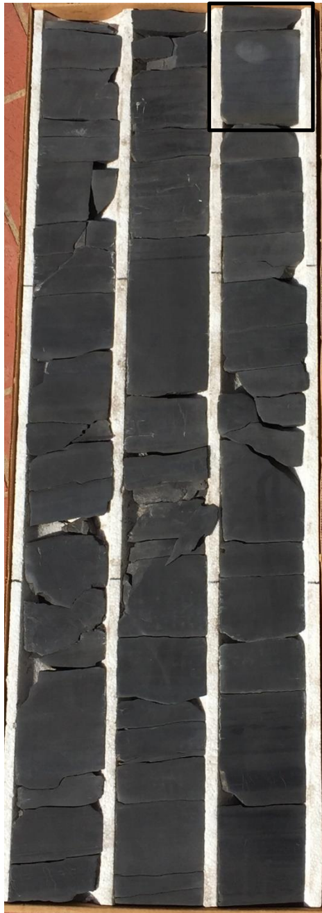
Appendix B. McDonald 2H-16E core photographs of subsea depths 6,277 feet to 6,268 feet (left figure). Depth shallows from bottom right corner to top left corner at a thickness of 3 feet per column in core box. Evident burrowing occurs within silica- and pyrite-rich laminae from 6,274.4 feet to 6,274 feet (upper right).
