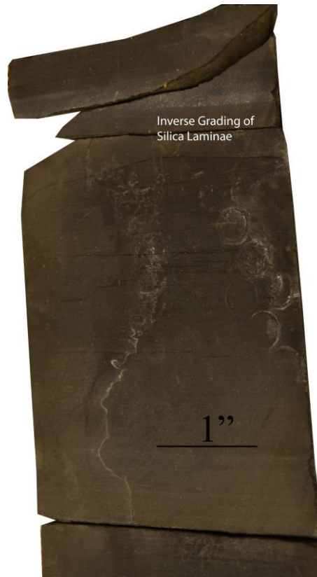
Appendix A. Williams 1H-7X core photographs of subsea depths 12,893 feet to 12,887 feet (left figure). Depth shallows from bottom right corner to top left corner at a thickness of 3 feet per column in core box. Inverse grading within silica-rich laminae in the A-SM lithofacies (upper right). Depth of 12,890.3 feet to 12,890 feet.
