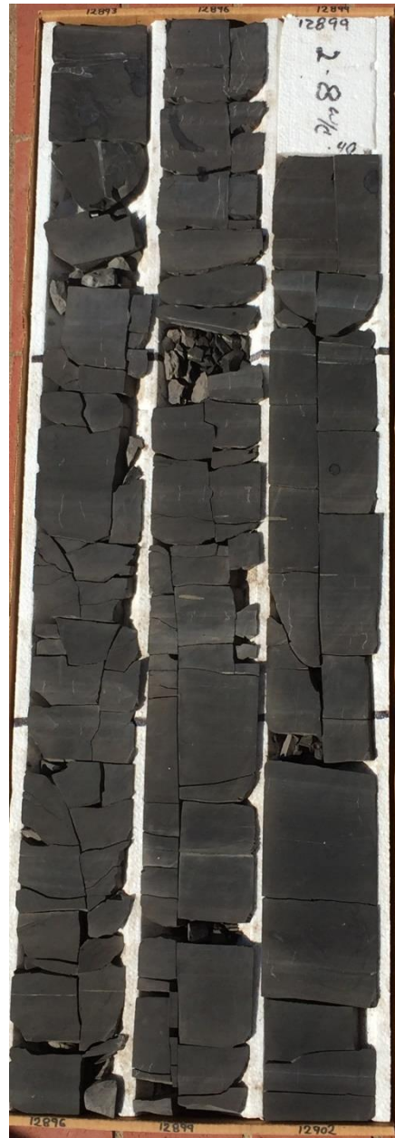
Appendix A. Williams 1H-7X core photographs of subsea depths 12,902 feet to 12,893 feet (middle figure). Depth shallows from bottom right corner to top left corner at a thickness of 3 feet per column in core box.
