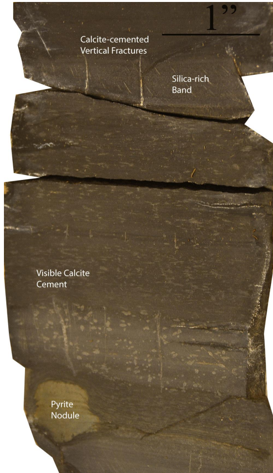
Appendix B. McDonald 2H-16E core photographs of subsea depths 6,310 feet to 6,301 feet (left figure). Base of SM lithofacies occurs at 6,306 feet. Depth shallows from bottom right corner to top left corner at a thickness of 3 feet per column in core box. Silica-cemented bands containing calcite-cemented vertical fractures and visible calcite cement and a pyrite nodule occur from 6,312.6 feet to 6,312.4 feet (upper right).
