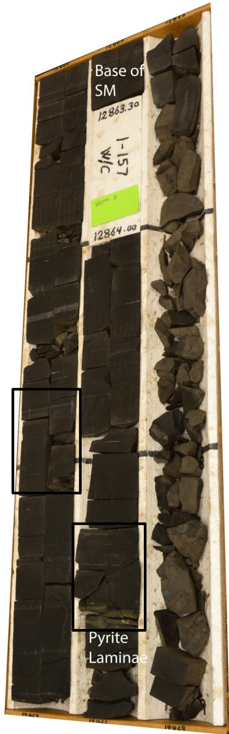
Appendix A. Williams 1H-7X core photographs of subsea depths 12,869 feet to 12,860 feet (left figure). Depth shallows from bottom right corner to top left corner at a thickness of 3 feet per column in core box. Pyrite laminae and inverse grading of silica-rich laminae occur from 12,865.8 feet to 12,865.4 feet in the A-SM lithofacies (upper right). Multiple silica-rich laminae containing calcite-cemented vertical fractures and inverse grading occurs from 12,862 feet to 12,861.7 feet in the SM lithofacies (bottom right).
