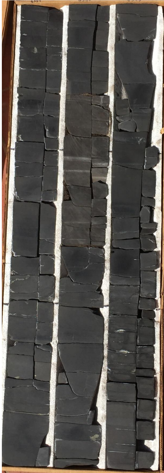
Appendix B. McDonald 2H-16E core photographs of subsea depths 6,346 feet to 6,337 feet (left figure). Depth shallows from bottom right corner to top left corner at a thickness of 3 feet per column in core box. Silt to sand-sized possible radiolarians exhibiting chalcedony chert with associated calcite cement occurs at 6,340.65 feet, XPL (upper right).
