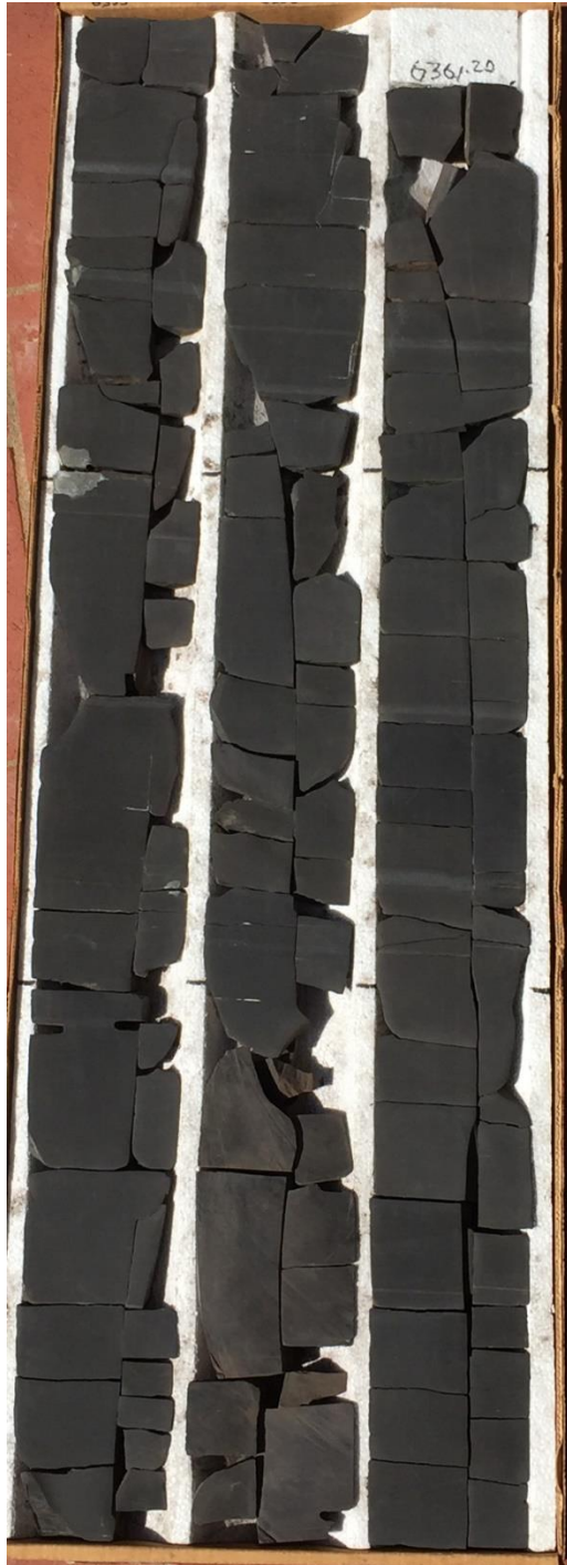
Appendix B. McDonald 2H-16E core photographs of subsea depths 6,364 feet to 6,355 feet (left figure). Depth shallows from bottom right corner to top left corner at a thickness of 3 feet per column in core box. Silt-sized detrital quartz lense surrounded by silt-sized detrital quartz and dolomite rhombs occurs at 6,360.2 feet, XPL (upper right).
