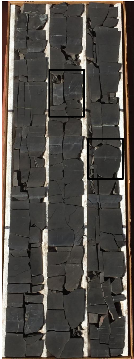
Appendix A. Williams 1H-7X core photographs of subsea depths 12,851 feet to 12,842 feet (left figure). Depth shallows from bottom right corner to top left corner at a thickness of 3 feet per column in core box. Possible burrow disrupting silica-rich laminae occurs from 12,849.6 feet to 12,849.4 feet in SM lithofacies (upper right). Two dolomite-cemented vertical fractures cause a horst and graben structure with silica-rich laminae. The silica-rich laminae also displays visible calcite cement. Image occurs from 12,846 feet to 12,845.7 feet (middle right).
