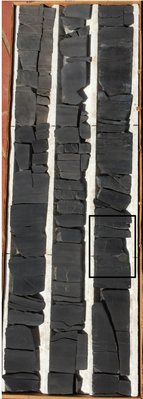
Appendix B. McDonald 2H-16E core photographs of subsea depths 6,310 feet to 6,301 feet (left figure). Base of SM lithofacies occurs at 6,306 feet. Depth shallows from bottom right corner to top left corner at a thickness of 3 feet per column in core box. Silica-cemented bands containing calcite-cemented vertical fractures and visible calcite cement and a pyrite nodule occur from 6,312.6 feet to 6,312.4 feet (upper right).
