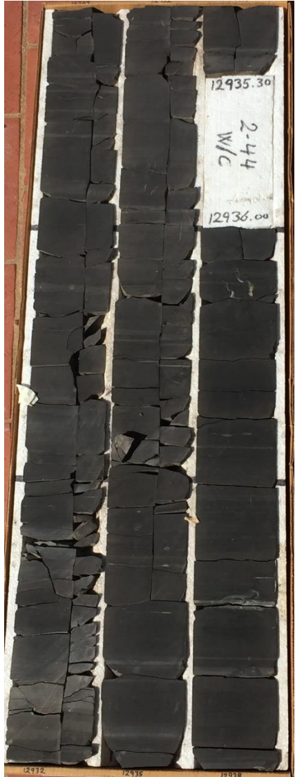
Appendix A. Williams 1H-7X core photographs of subsea depths 12,938 feet to 12,929 feet (left figure). Depth shallows from bottom right corner to top left corner at a thickness of 3 feet per column in core box. A cluster of silt to very fine sand-sized possible radiolarians surrounded in a clay-rich lithology in the A-SM lithofacies. Depth at 12,935 feet, PPL.
