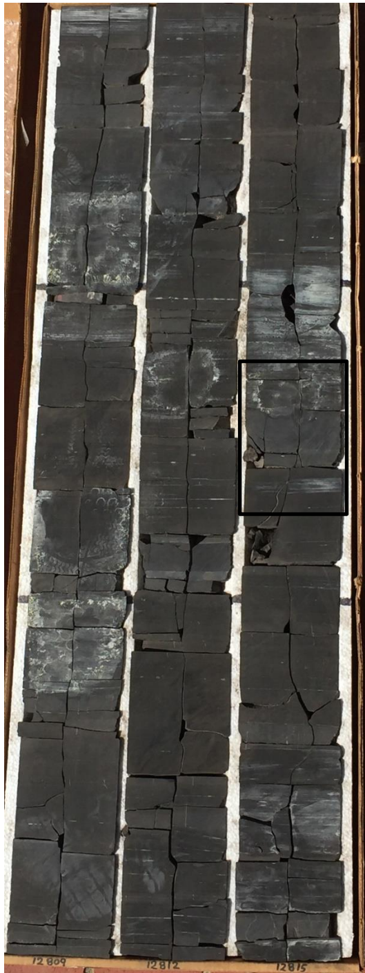
Appendix A. Williams 1H-7X core photographs of subsea depths 12,815 feet to 12,806 feet (left figure). Depth shallows from bottom right corner to top left corner at a thickness of 3 feet per column in core box. Silica-cemented band containing open vertical and sub-parallel fractures as well as silica-rich laminae occurs from 12,813.6 feet to 12,813.4 feet (upper right).
