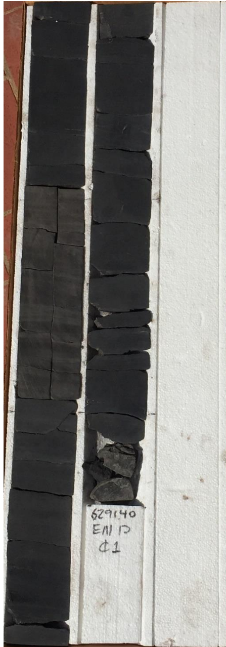
Appendix B. McDonald 2H-16E core photographs of subsea depths 6,291.4 feet to 6,286 feet (middle figure). Depth shallows from bottom right corner to top left corner at a thickness of 3 feet per column in core box.
