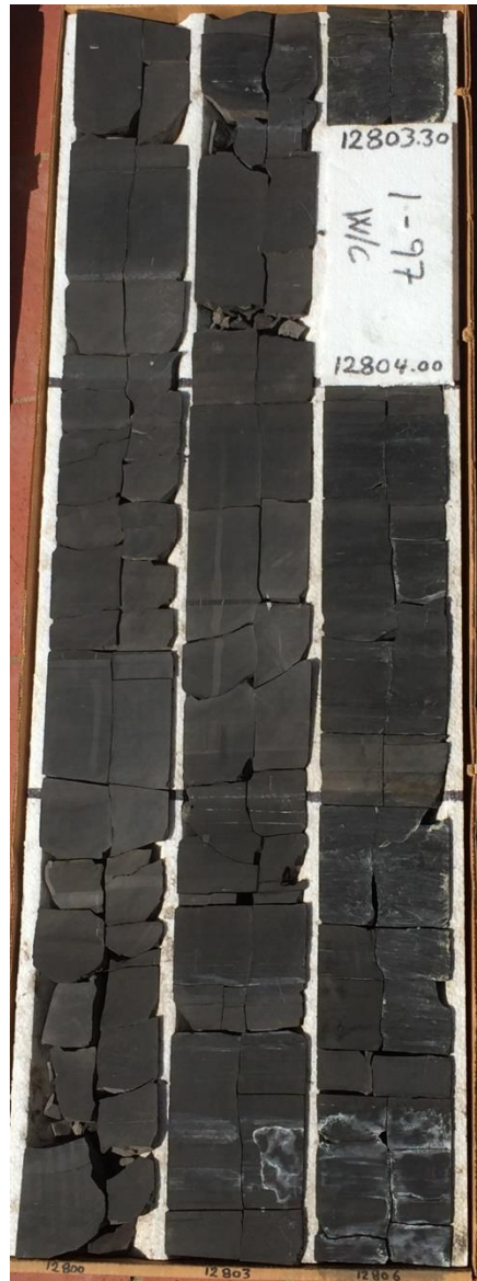
Appendix A. Williams 1H-7X core photographs of subsea depths 12,806 feet to 12,797 feet (middle figure). Depth shallows from bottom right corner to top left corner at a thickness of 3 feet per column in core box.
