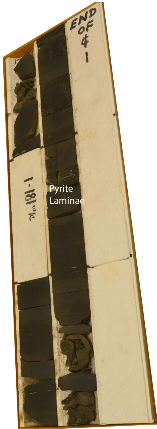
Appendix A. Williams 1H-7X core photographs of subsea depths 12,893 feet to 12,887 feet (left figure). Depth shallows from bottom right corner to top left corner at a thickness of 3 feet per column in core box. Inverse grading within silica-rich laminae in the A-SM lithofacies (upper right). Depth of 12,890.3 feet to 12,890 feet.
