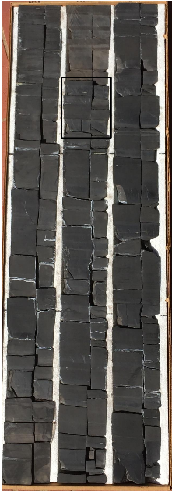
Appendix B. McDonald 2H-16E core photographs of subsea depths 6,337 feet to 6,328 feet (left figure). Base of SM lithofacies occurs at 6,337 feet. Depth shallows from bottom right corner to top left corner at a thickness of 3 feet per column in core box. Abundant silica-cemented bands containing numerous calcite-cemented ptymatic fractures occur from 6,331.8 feet to 6,331.5 feet (upper right).
