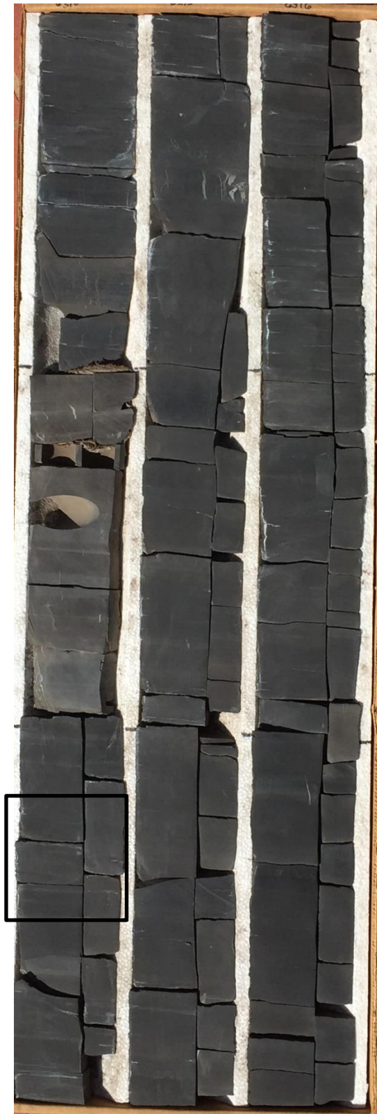
Appendix B. McDonald 2H-16E core photographs of subsea depths 6,319 feet to 6,310 feet (left figure). Depth shallows from bottom right corner to top left corner at a thickness of 3 feet per column in core box. Silica-rich laminae containing a micro fault occurs from 6,312.5 feet to 6,312.4 feet (upper right). Abundant silt to sand-sized possible radiolarians occur at 6,311 feet, PPL (middle right).
