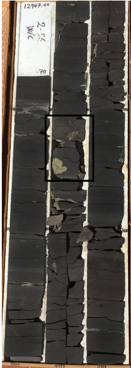
Appendix A. Williams 1H-7X core photographs of subsea depths 12,956 feet to 12,947 feet (left figure). Depth shallows from bottom right corner to top left corner at a thickness of 3 feet per column in core box. Upper right figure shows pyrite nodules and open fractures in the A-SM lithofacies. Depth of 12,951.5 feet to 12,951 feet.
