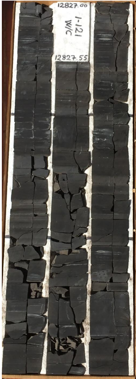
Appendix A. Williams 1H-7X core photographs of subsea depths 12,833 feet to 12,824 feet (left figure). Depth shallows from bottom right corner to top left corner at a thickness of 3 feet per column in core box. Possible silt-sized white radiolarian surrounded by tasmanites cysts that have been mineralized by phosphate occurs at 12,831.35 feet, PPL (upper right).
