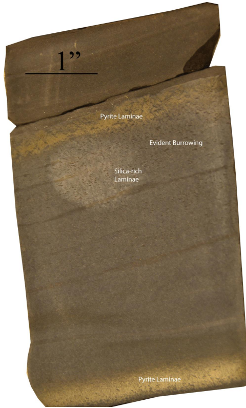
Appendix B. McDonald 2H-16E core photographs of subsea depths 6,277 feet to 6,268 feet (left figure). Depth shallows from bottom right corner to top left corner at a thickness of 3 feet per column in core box. Evident burrowing occurs within silica- and pyrite-rich laminae from 6,274.4 feet to 6,274 feet (upper right).
