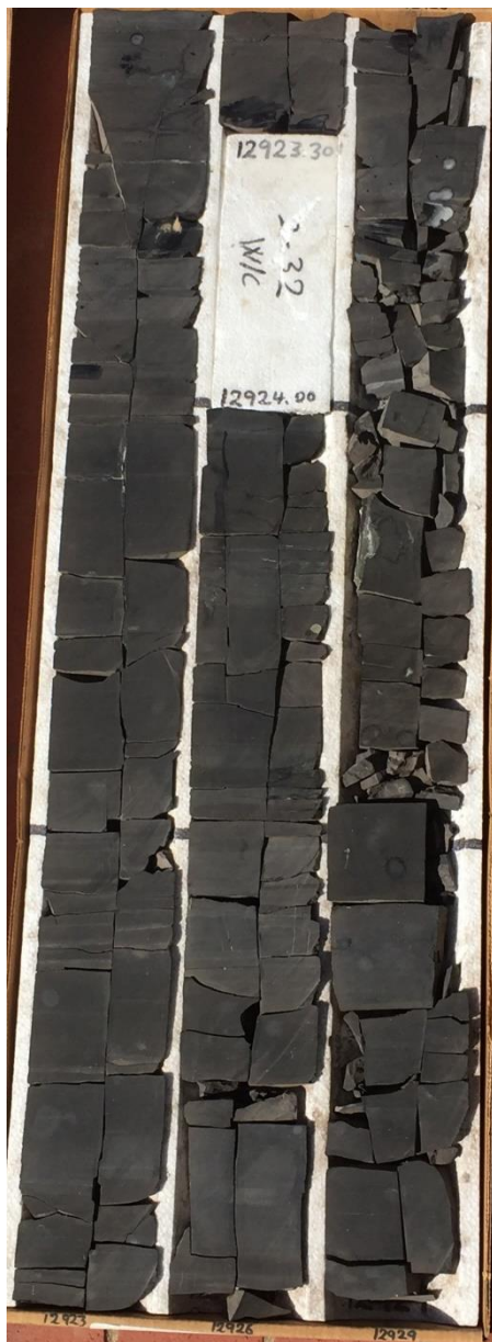
Appendix A. Williams 1H-7X core photographs of subsea depths 12,929 feet to 12,920 feet (middle figure). Depth shallows from bottom right corner to top left corner at a thickness of 3 feet per column in core box. Ripple mark near 12,924 feet.
