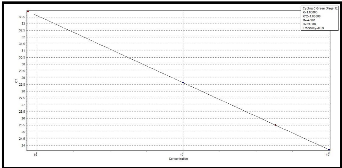
Fig.11B. Standard Curve of figure 11A. The standard curve shows threshold cycle (Ct) on the y-axis and the DNA concentration on the x-axis. Slope, y-intercept, and correlation coefficient values shows the performance of this reaction. R^2 = 1 reflects the linearity of the standard curve. M measures the reaction efficiency, equivalent to -3.32 for 100% efficiency.
