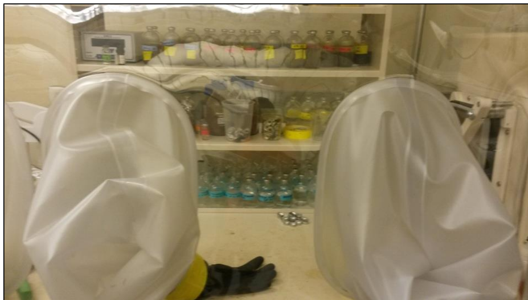
Figure 96: The Coy Labs glove box is a sealed container used to create a separate atmospheric environment for specific microbial growth. The microcosms are placed in a separate vacuum box, in order to remove the oxygen-containing air and replace it with an anaerobic nitrogen air mixture. This glove box is used to grow anaerobic microbial cultures.
