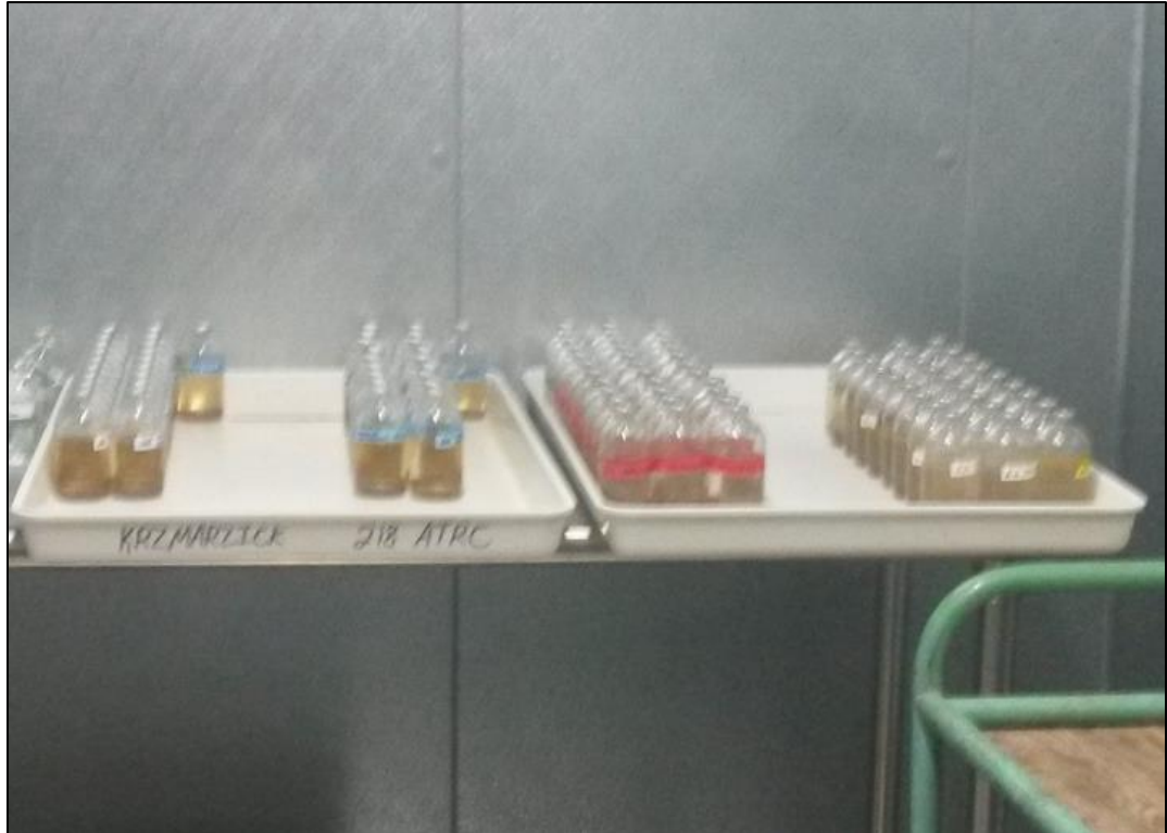
Figure 95: Microcosms were stored in a Norlake Scientific incubator. The incubator was used to maintain an optimal temperature and humidity for microbial growth. The incubators temperature was set to 30 °C.
