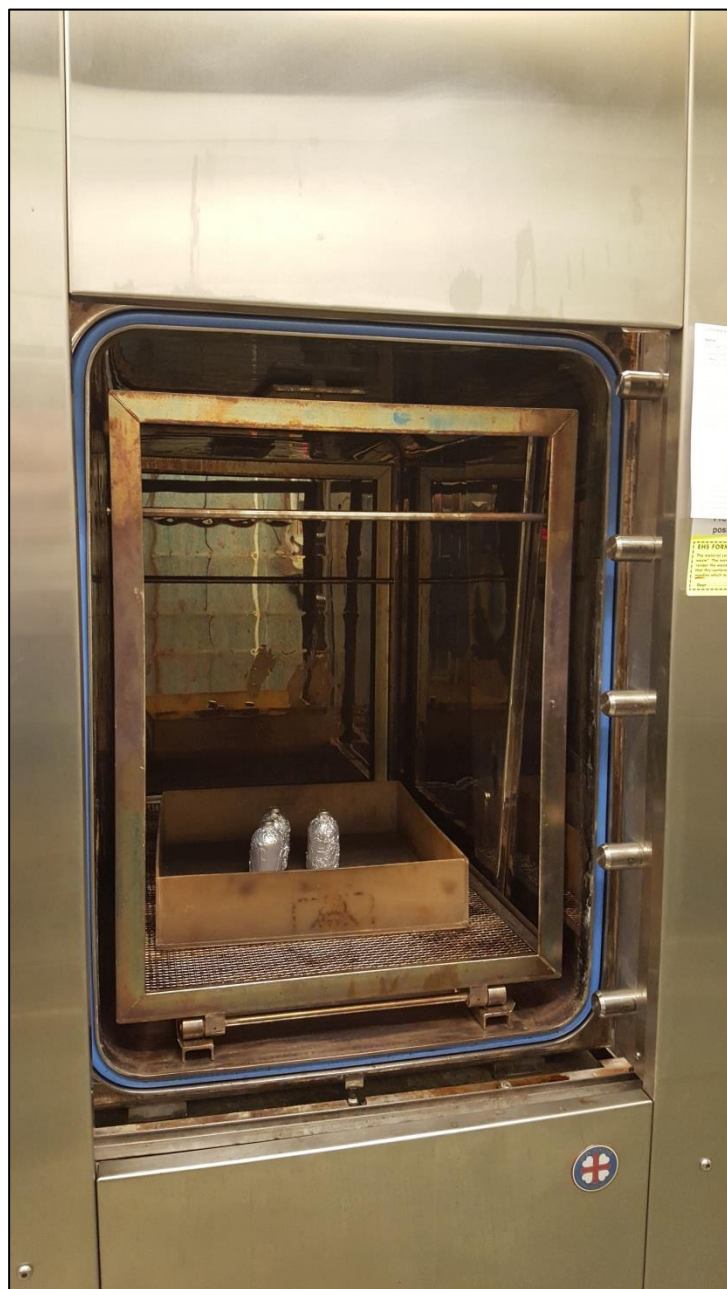
Figure 97: The Primus Sterilizer Co. Inc. autoclave is a chamber that raises the temperature and pressure in order to sterilize its contents. The autoclave runs cycles reaching temperatures of 250 °F and 18 psig. Microcosms were placed in an autoclave cycle once a day, three days in a row to ensure the removal of microbial activity. These controls allow conclusions to be made about how the benzene and toluene are being removed from the microcosm system.
