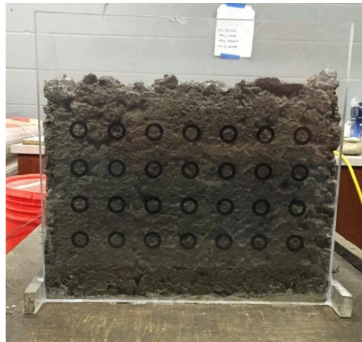
Figure 2. 10: The point count template positioned in front of a concrete side.
