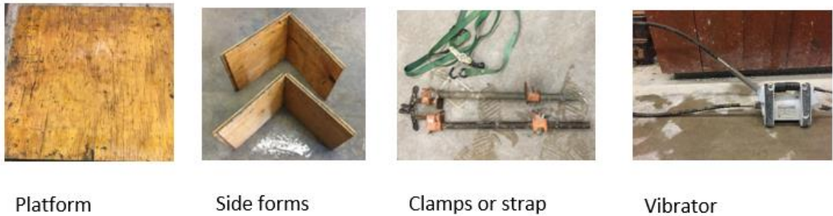
Figure 2. 1: The Box Test components.
