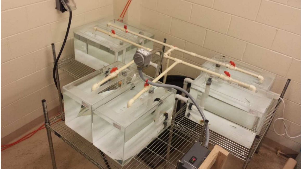
Figure 2. Sump system for testing critical thermal maximum (CTM). A pump discharges water into the 37.85-L aquariums and a gravity fed system discharges water into the 189.27-L sump. Water is heated in the sump by a 5000-W Smartone heater (OEM Heaters, Saint Paul, MN).
