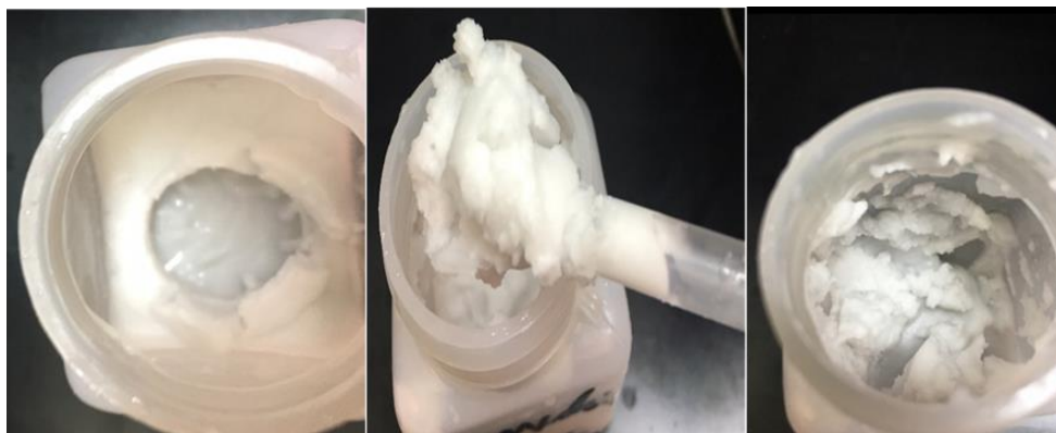
Figure 6.2: Visual confirmation of hydrate formation in 40 wt.% water-in-oil emulsion containing wax and surfactant in the oil phase
