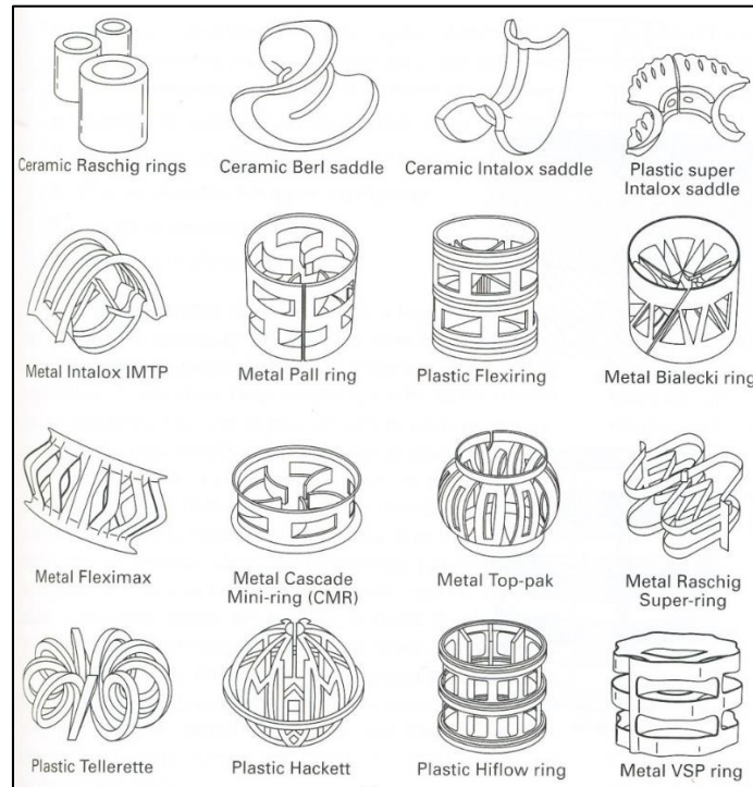
Figure 3.2. Typical random packing shapes for packed columns. Figure reprinted from Seader et al. (2006) with permission from the publisher. Copyright© 2011, 2006, 1998 JohnWiley & Sons, Inc. All rights reserved.
