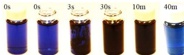
Figure 7- 8. Changing color during sensing of 35% H_2O_2 solution as a function of time using the blue reagent
