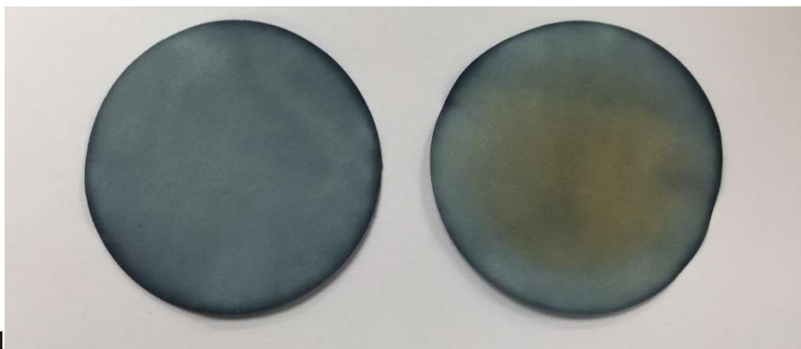
Figure 7- 6. Paper with vanadyl oxalate solution: as manufactured (left); exposed to hydrogen peroxide vapors (right)
