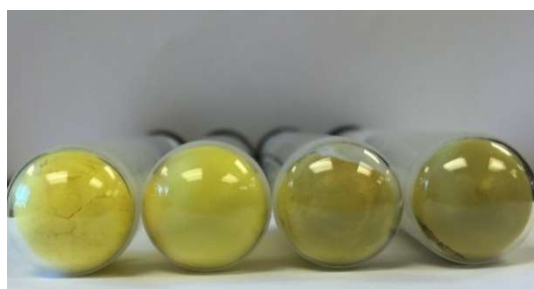
Figure 2- 10. Color change of tungstic acid reaction with stilbene for one day at different temperatures; from the left to the right: bright yellow (R.T.), pale yellow (100 °C), light greenish yellow (120 °C), and light green (150 °C)
