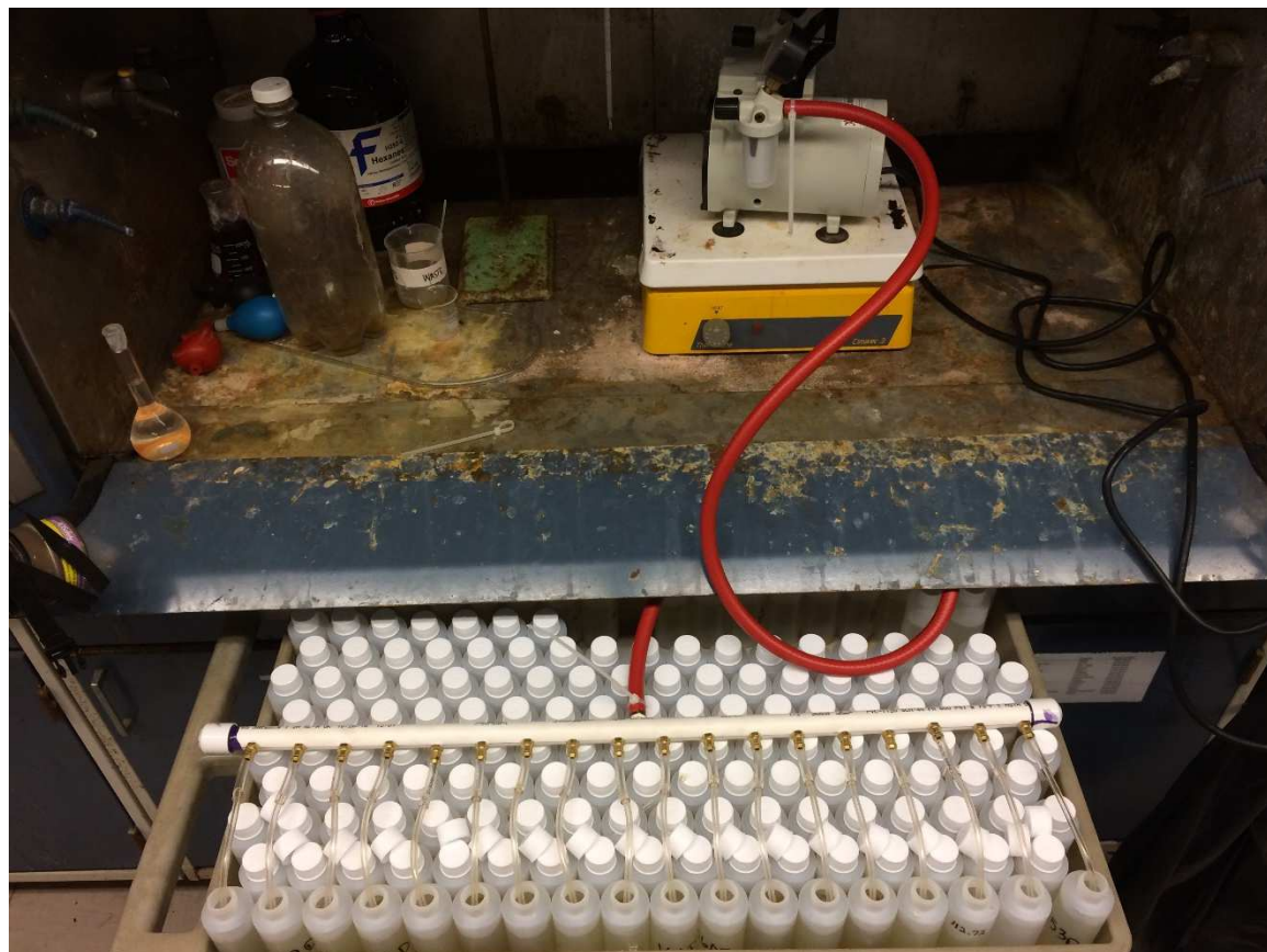
Figure 2.1. Picture of air pump and manifold built in house to aerate Extraction D samples and oxidize residual sodium dithionate. During operation, air was bubbled through a large flask with water to reduce evaporation in the samples.
