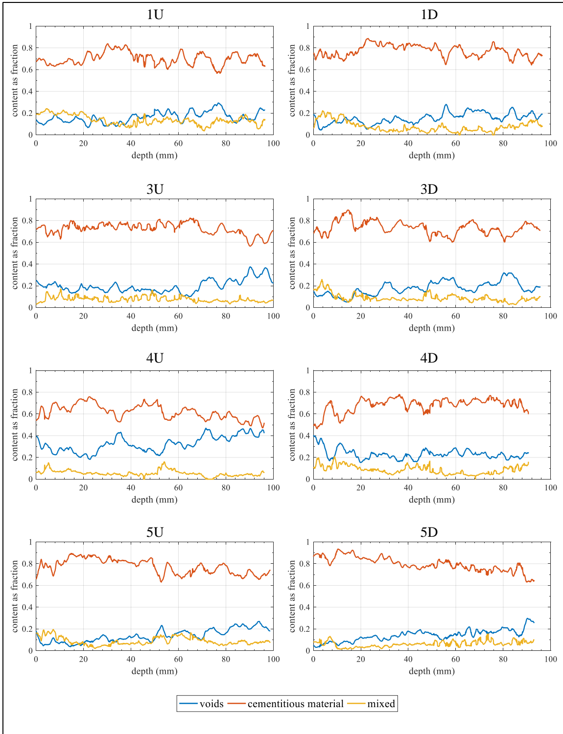
Figure 5.9. Void, mixed, and cementitious material component fractions with depth for cores 1U, 1D, 3U, 3D, 4U, 4D, 5U, and 5D from Hsieh et al. (1998) methodology. The top surface of the core is at 0 mm.
