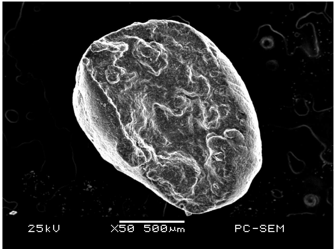
Figure 4.2 SEM micrograph showing the cross-sectional morphology of spirulina–alginate beads made with external gelation process with alginate 1% and \text{CaCl}_2 15%.
