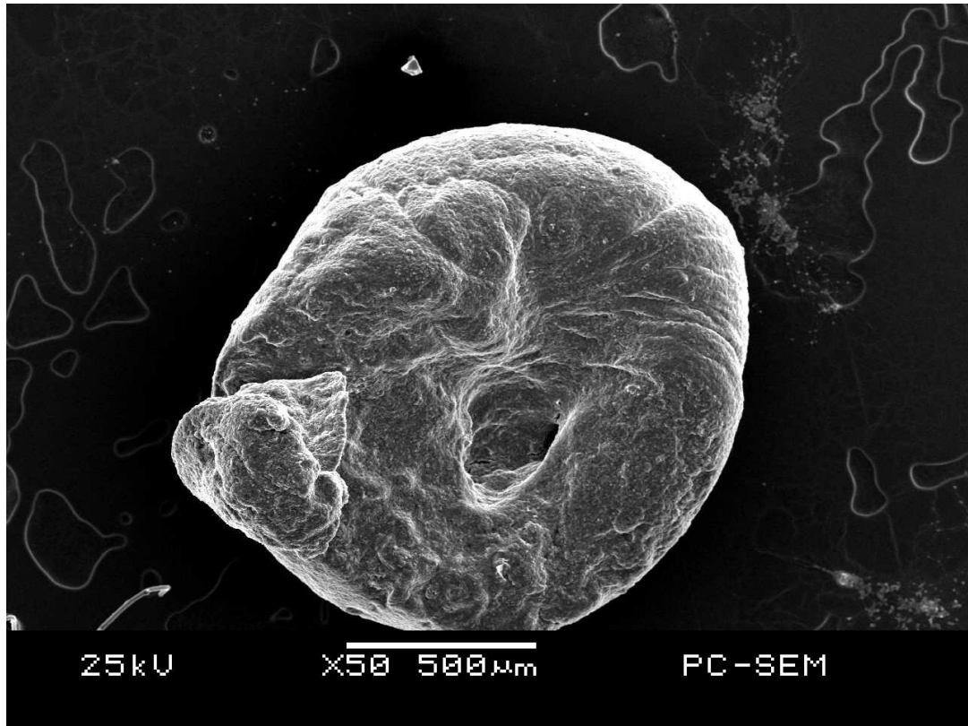
Figure 4.1 SEM micrograph showing the cross-sectional morphology of spirulina–alginate beads made with external gelation process with alginate 1% and \text{CaCl}_2 10% .
