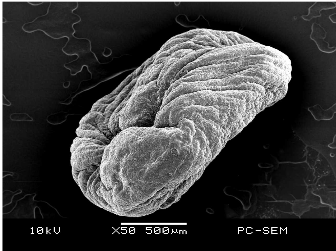
Figure 4.7 SEM micrograph showing the exterior morphology of spirulina-alginate beads made with external gelation process with alginate 1% and \text{CaCl}_2 10%.
