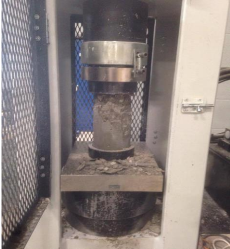
Figure 3.4 Compressive strength testing
