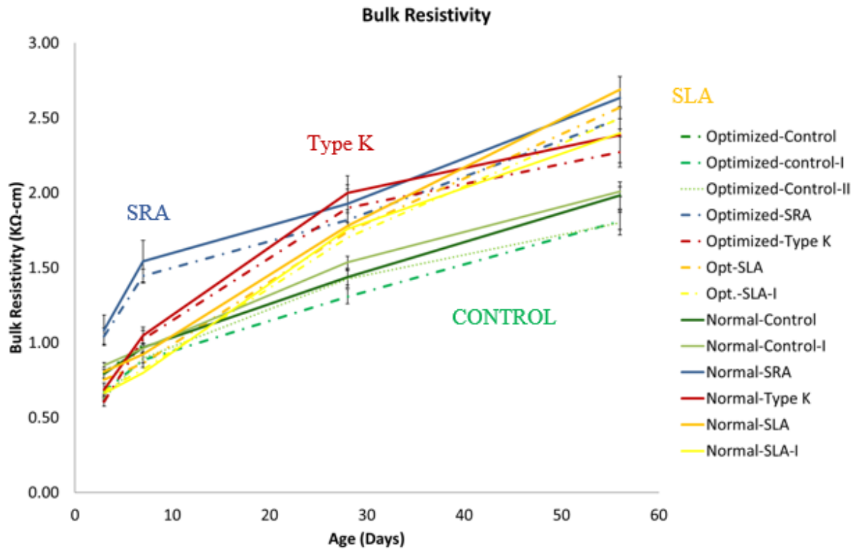
Figure 6.6 Bulk resistivity change over time for the different mixtures.
