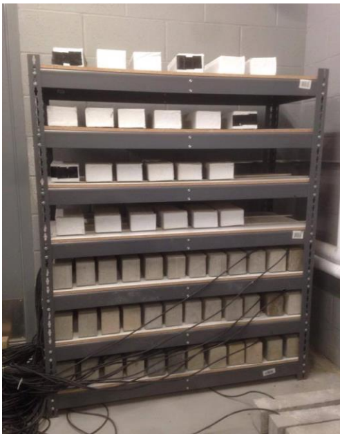
Figure 3.2 drying arrangement for all axial beams and curling beams
