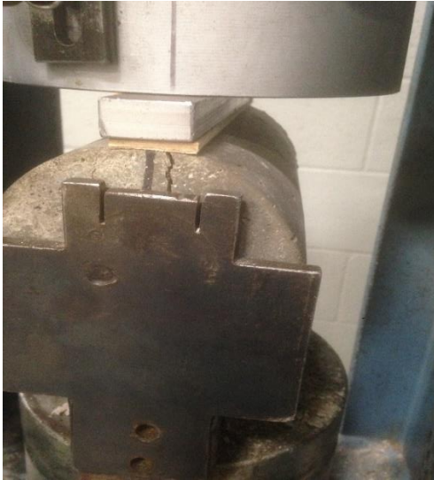
Figure 3.5 Splitting Tensile Test
