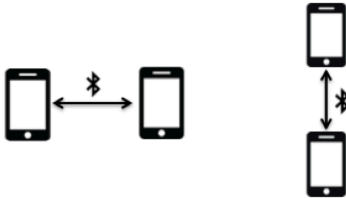
Figure 4.2: Side-Side and top-bottom placement of devices
