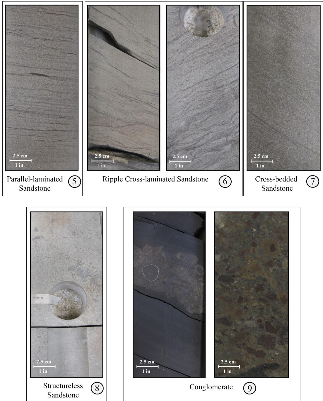
Figure 8. Core-defined lithofacies include 1) coal, 2) organic claystone, 3) laminated and bioturbated claystone, 4) poorly-bedded heterolithic sandstone, 5) parallel-laminated sandstone, 6) ripple cross-laminated sandstone, 7) cross-bedded sandstone, 8) structureless sandstone, and 9) conglomerate.
