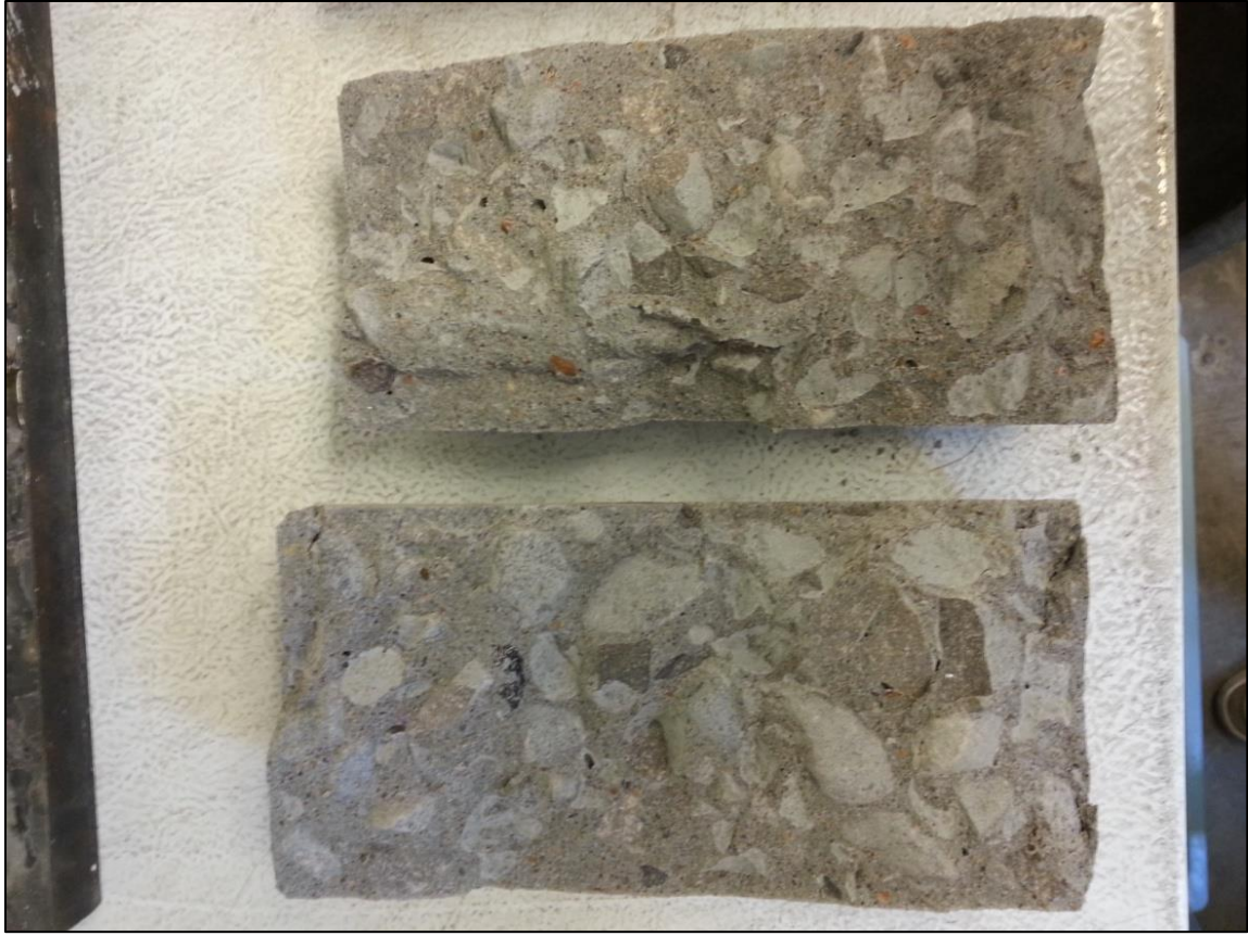
Figure 19: Example of failure in the concrete aggregates instead of the paste
