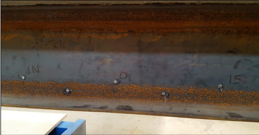
Figure 10: DEMEC points location on the web of the steel girder for Porotype Beam 1
