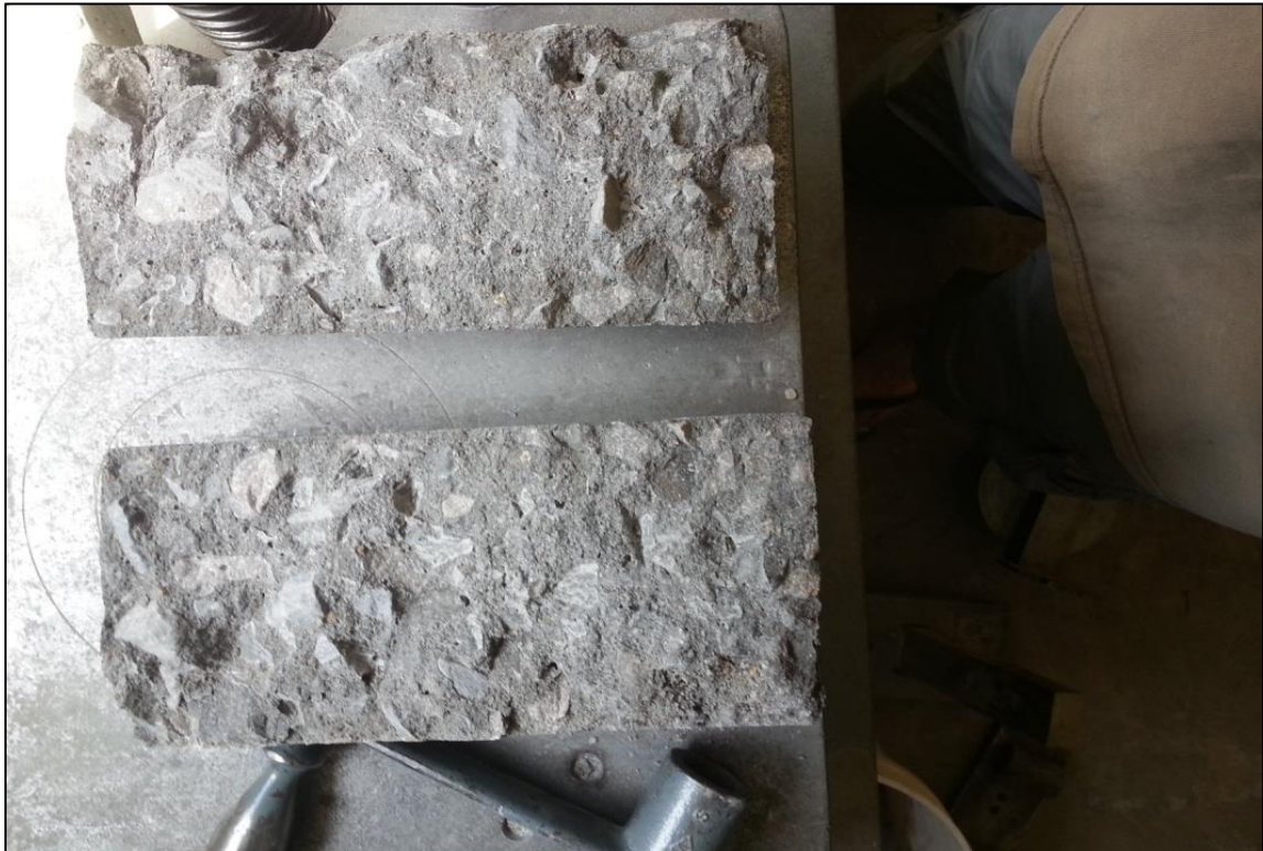
Figure 18: Example of failure in the concrete paste instead of the aggregates
