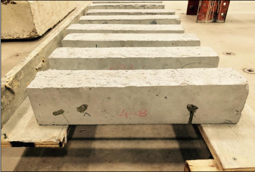
Figure 21: Transverse view of unrestrained shrinkage prisms for Prototype Beam 1 and 2
