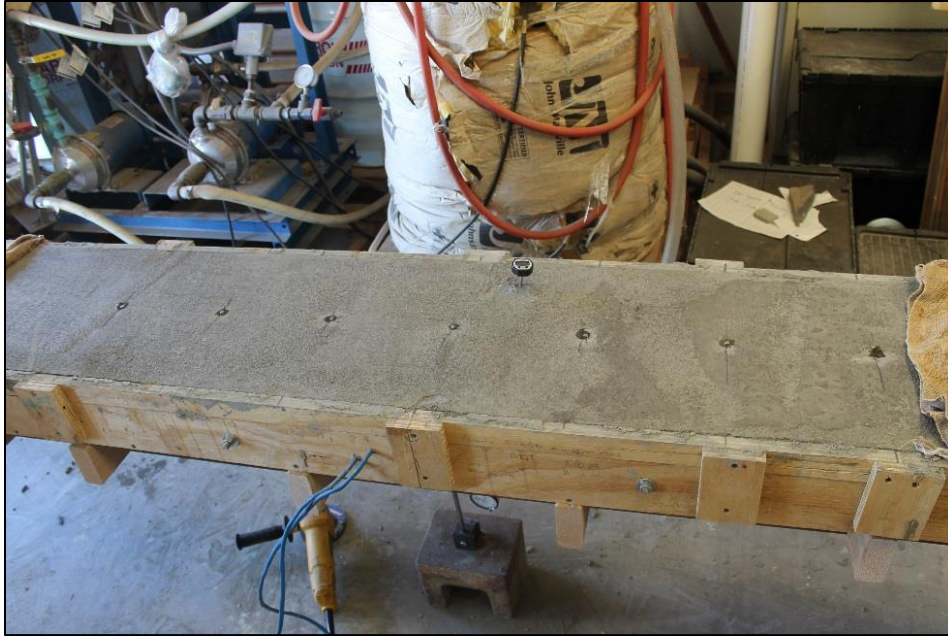
Figure 8: DEMEC points to measure strains and thermocouples and thermometer to measure temperature variance.
