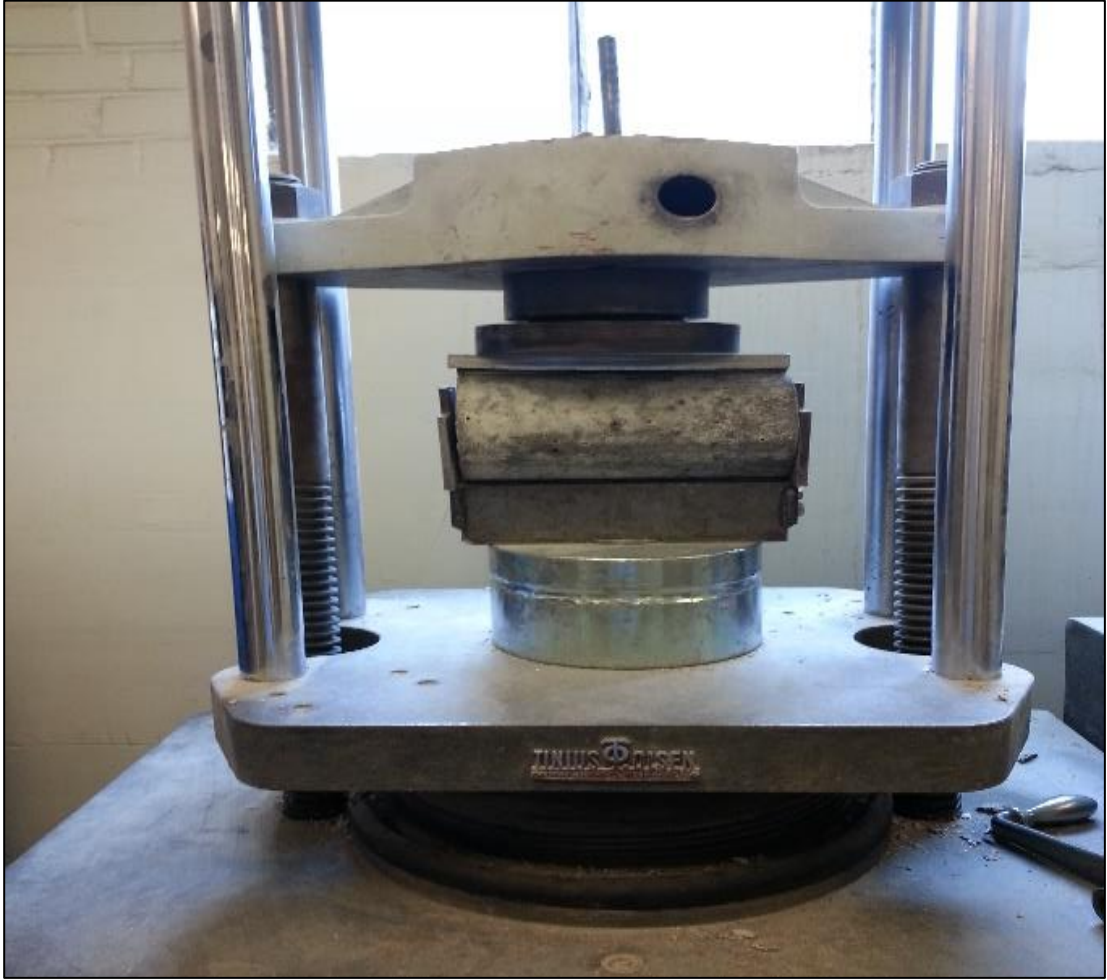
Figure 14: Splitting cylinder tensile strength test setup (ASTM C496)
