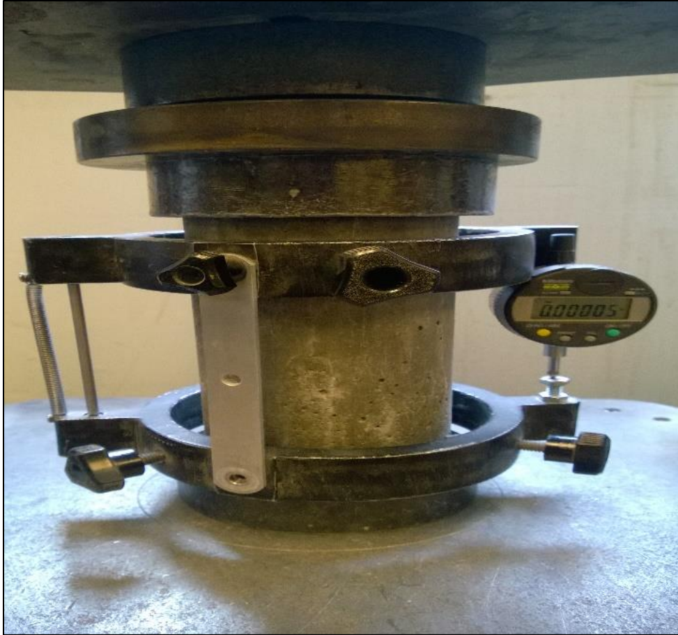
Figure 15: Measurement of the modulus of elasticity (ASTM C469)
