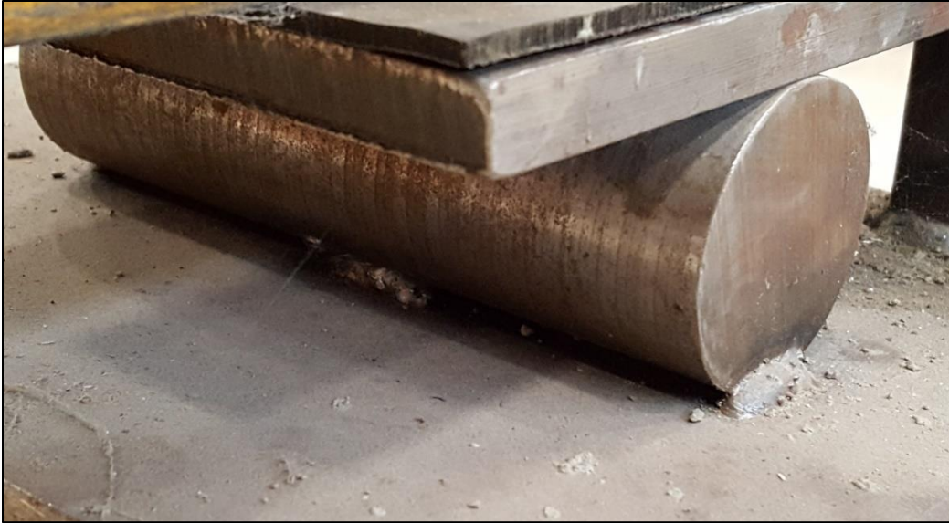
Figure 6: Welded pin support on the prototype beams
