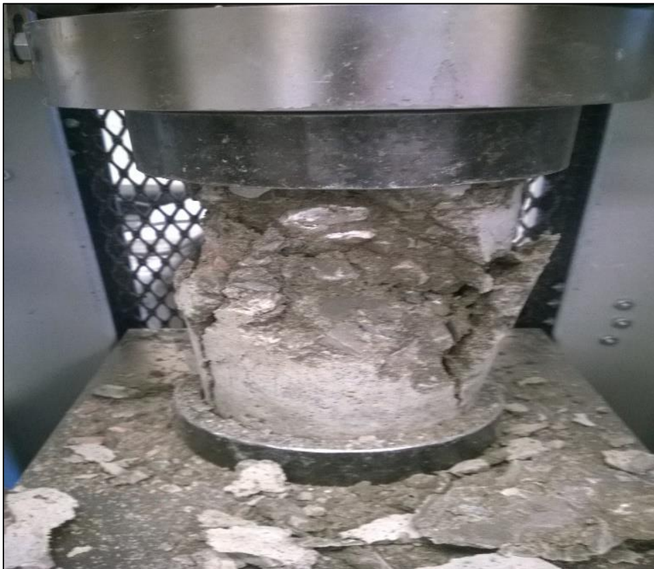
Figure 13: Concrete cylinder exhibiting a crushing failure (ASTM C39)
