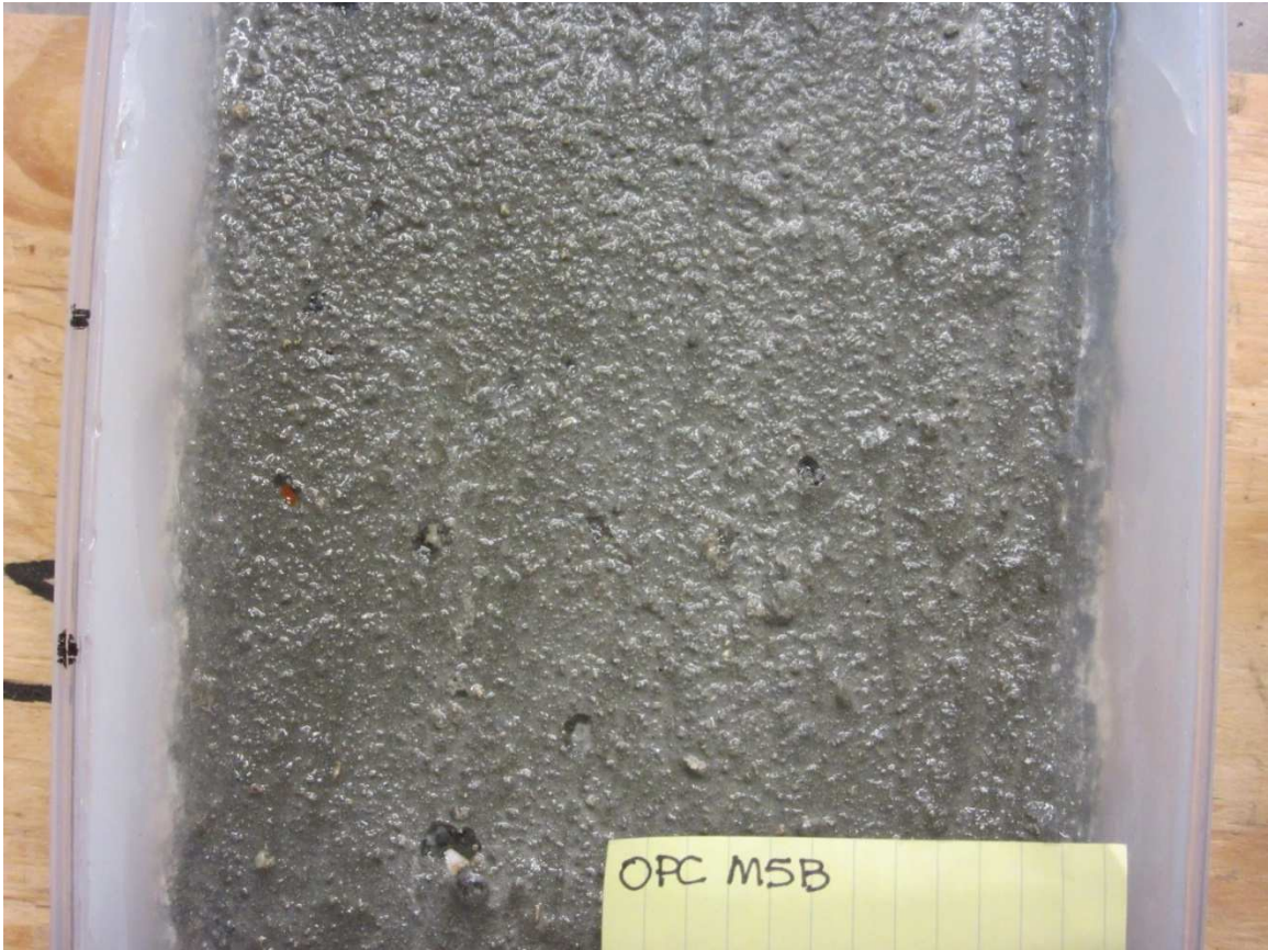
Figure 8: OPC Sample with Visual Rank of 1
