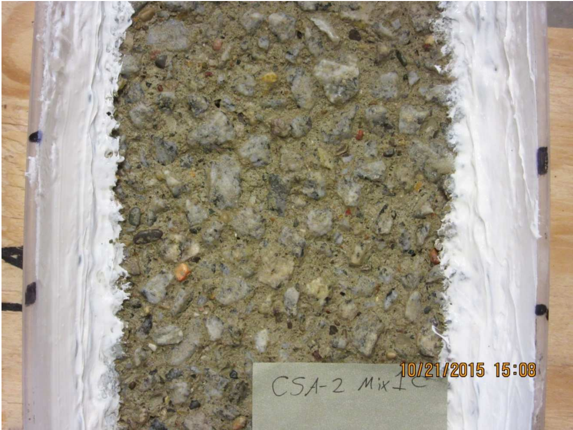
Figure 10: CSA2 Sample with Visual Rank of 5
