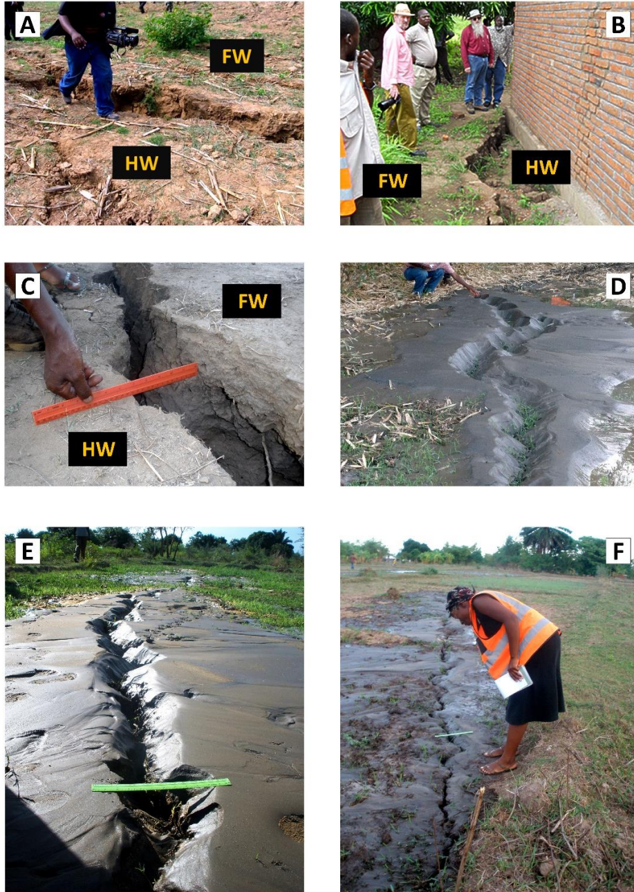
Figure 3. Photographs showing coseismic surface deformation associated with the ruptured fault of the 2009 Karonga earthquake. (a - b) Coseismic surface ruptures with normal-faulting style of displacement. HW = hanging wall, FW = foot wall. (c) Coseismic surface rupture with 13 cm lateral opening and 9 cm vertical offset. (d) Coseismic surface ruptures with sand blows.
