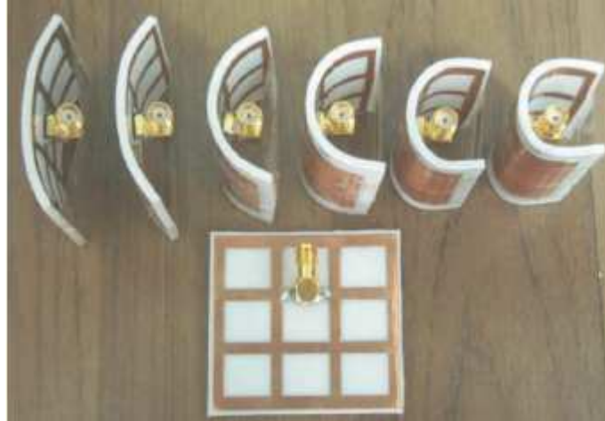
Figure 12 Bent patch antennas. Each is approximately 45 mm square. [8]
