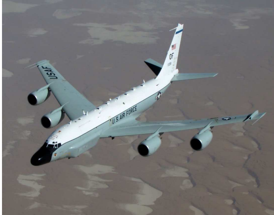
Figure 6 USAF RC-135 electronic surveillance aircraft. Note the cheek antenna fairings and the blade antennas along the spine and at the wingtips. Source: AF.mil
