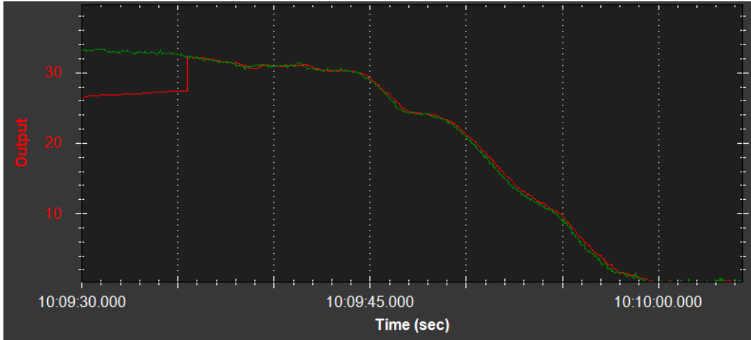
Figure 4.3: Anaconda Auto Land Performance, EKF Height Estimate and Laser Rangefinder State Time Trace [meters]
