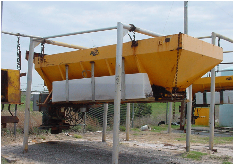
Figure 2. Hopper Type Spreader with Polyethylene Anti-icing Tanks
