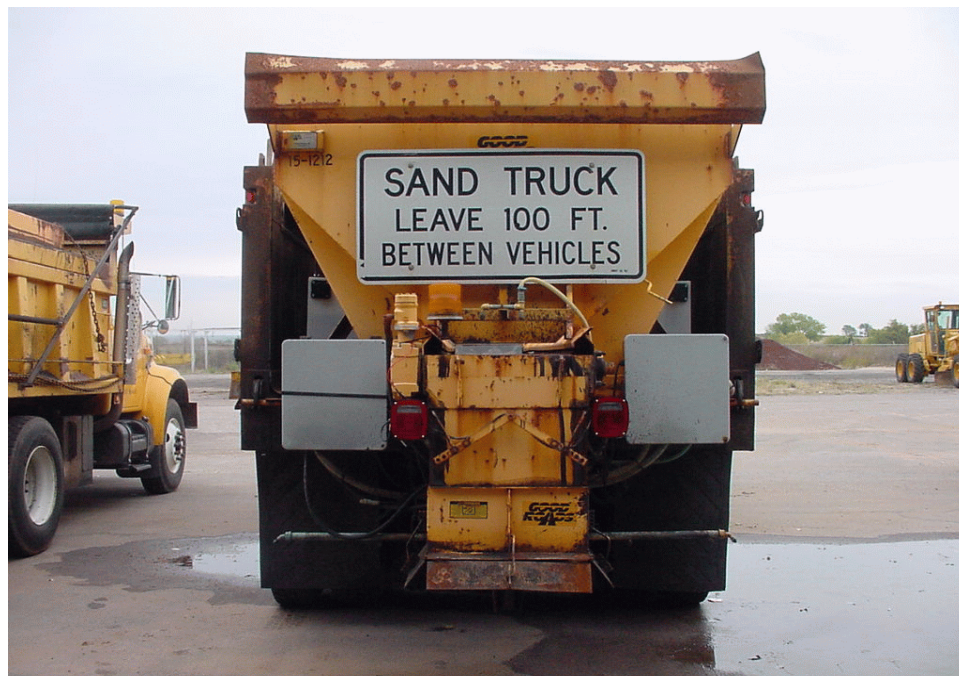
Figure 3. Mounted Hopper Type Spreader with Polyethylene Anti-icing Tanks
