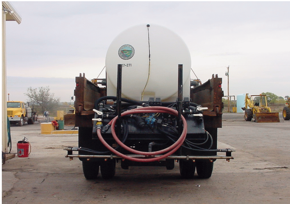
Figure 5. Truck Mounted Mobile Anti-icing System
