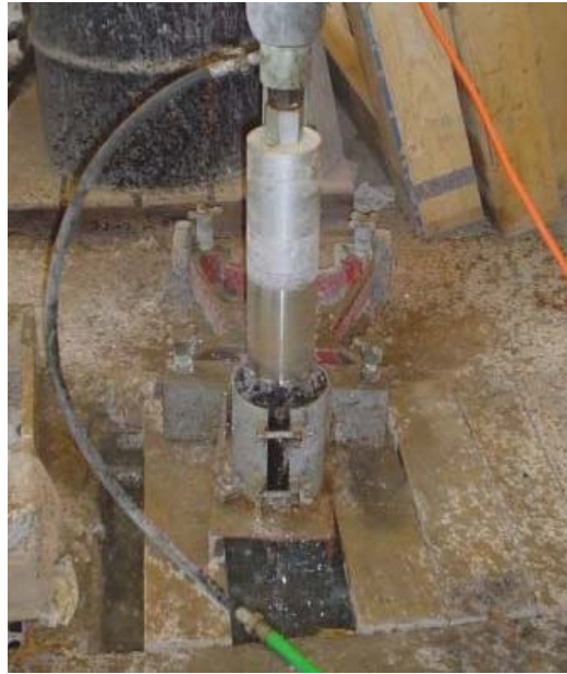
Figure 4 Sample being cored to required test diameter.
