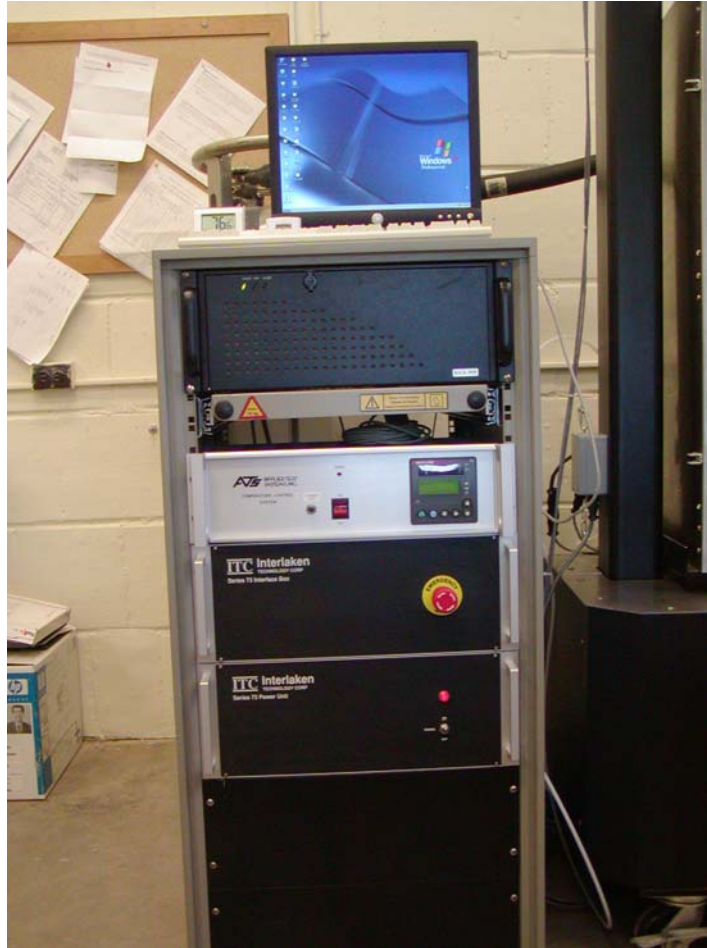
Figure 9 Control unit for the ITC dynamic modulus machine.
