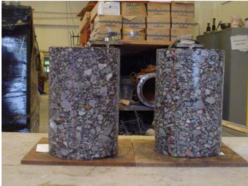
Figure 6 Test specimens for dynamic modulus testing.
