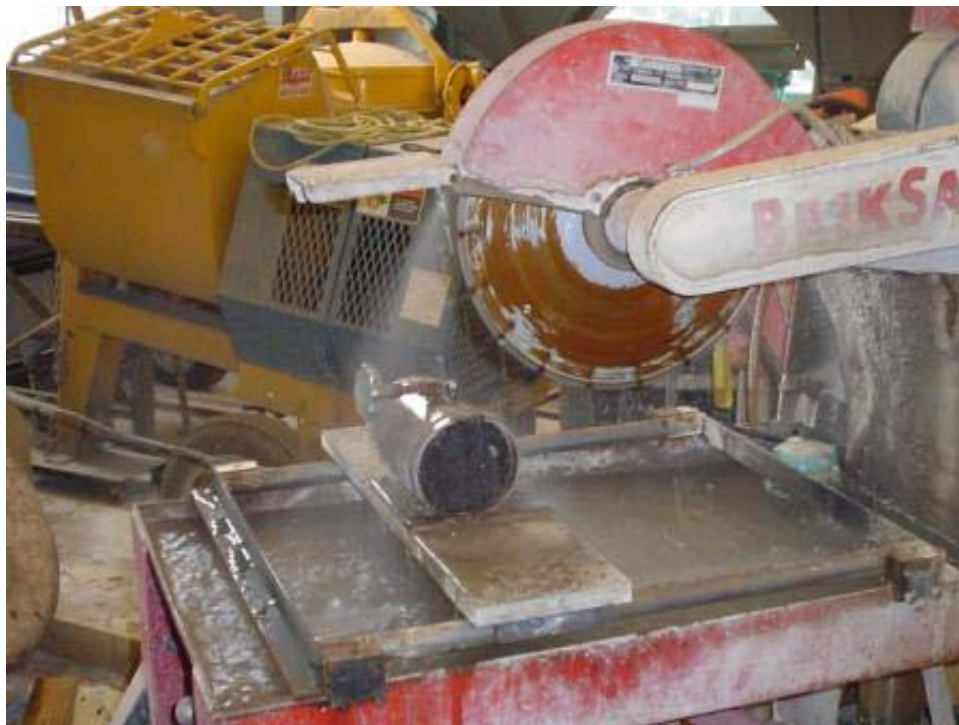
Figure 5 Sample being sawed to obtain parallel faces.
