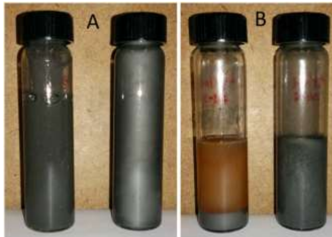
Figure 5.9. Suspendability of zero valent iron particles (2 \mu\text{m} ) by viscoelastic fluid. a. samples right after vortex mixing; b, samples after 10 minutes of centrifugation at 537 relative centrifugal force (RCF). Left vial, 26 wt% of zero valent iron in 2 wt% C 8 P 4 E 1 solution; right vial, 26 wt% of zero valent iron in viscoelastic fluid (2 wt% C 8 P 4 E 1 with 3.0 vol% oil).
