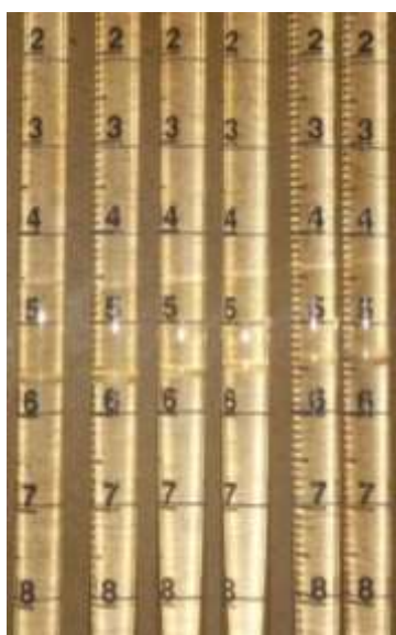
Figure 5.2. Winsor III microemulsion of 2 wt% C_8P_4E_1 /Isopar at NaCl concentration from 18.4 - 19.9 wt%
