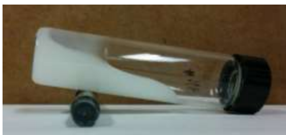
Figure 5.4. Viscous emulsion formed by 3 vol% of Isopar with 2 wt% C 8 P 4 E 1 solution at 19 wt% NaCl.
