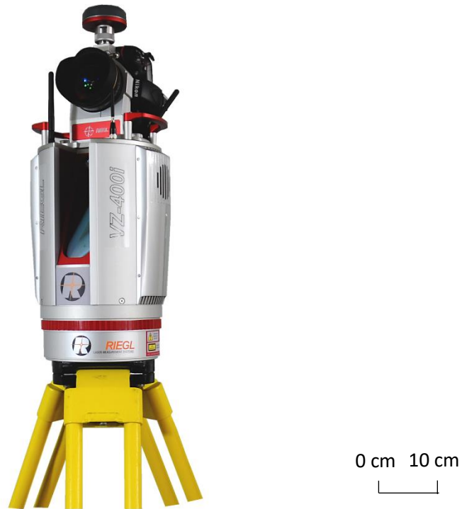
Figure 6: The REIGL® VE-400i 3D terrestrial LiDAR used in this study with Nikon camera attached to the top. The yellow part is the tripod at the bottom.
