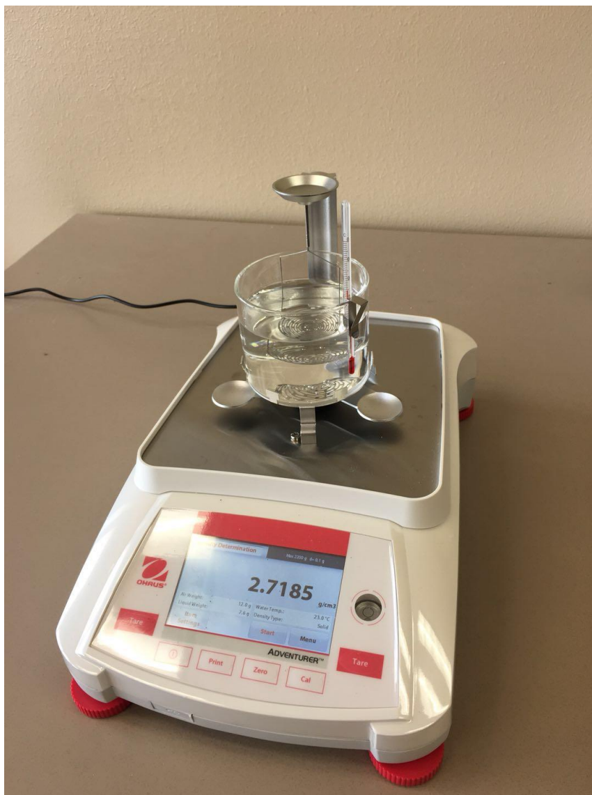
Figure 11: Ohaus Adventure Balance with density measurement kit.
