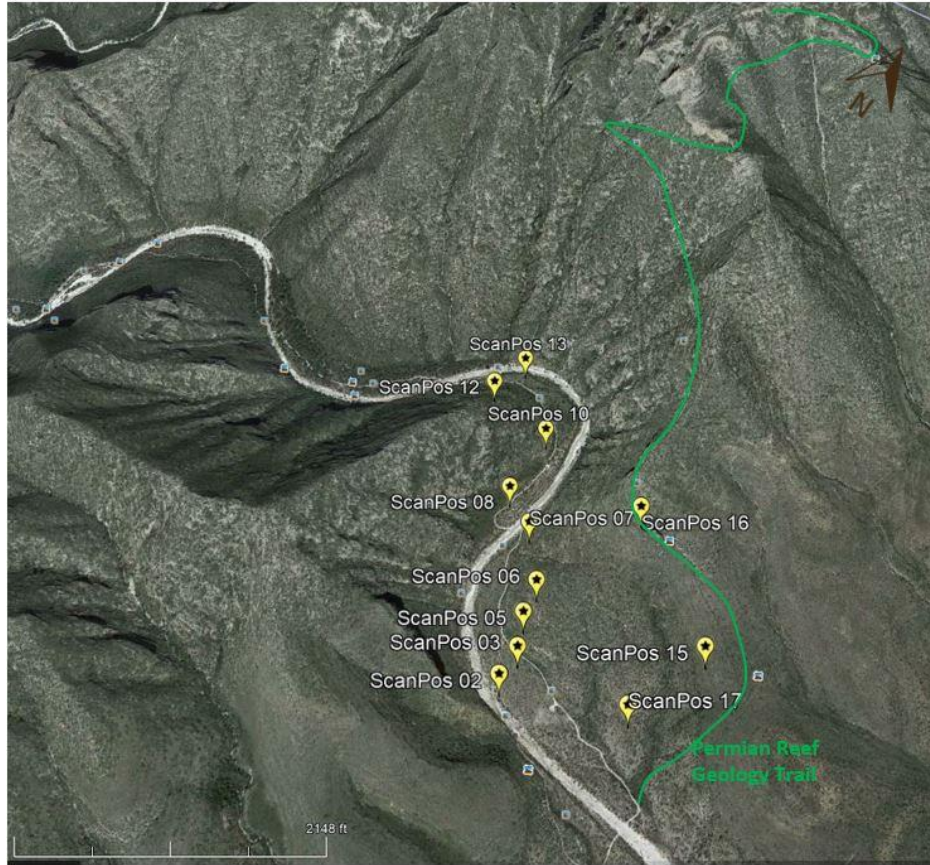
Figure 7: LiDAR scan position on Google Earth looking straight down into the canyon. Scans positions are marked in yellow.
