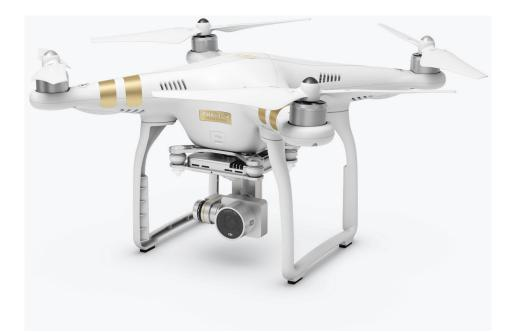
Figure B-1. The DJI Phantom 3 drone (shown here) was used for imaging the Burro Canyon Formation. Camera is f/2.8 with 940 field of view and 3-axis gimbal.
