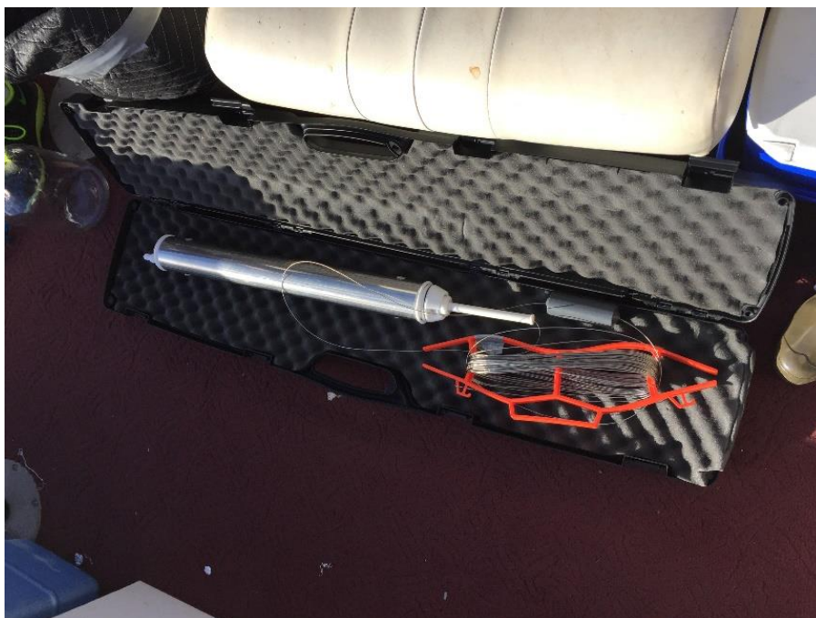
Figure 8. Stainless Steel 1.2 L Kemmerer water sampler.
