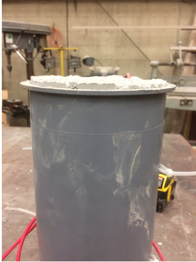
Figure 49: Visible height expansion of sample *ST210
