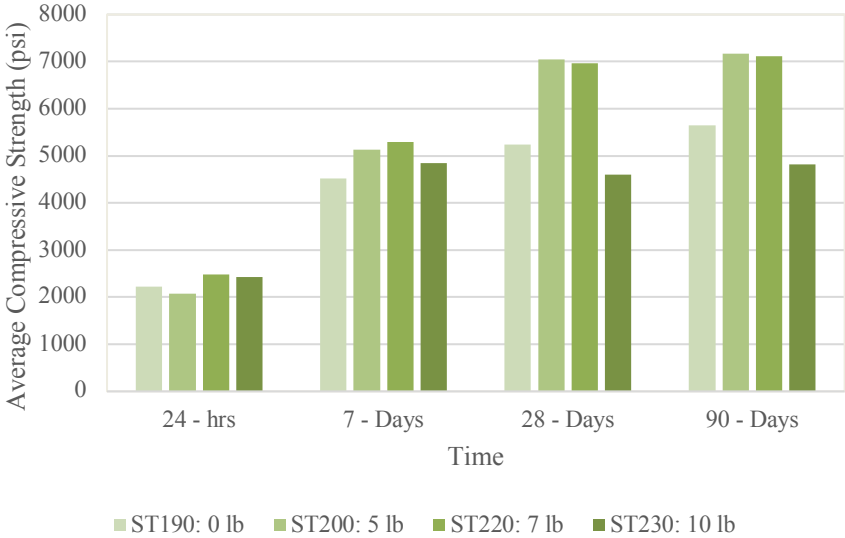
Figure 16: Average compressive strengths for Komponent® cement samples
