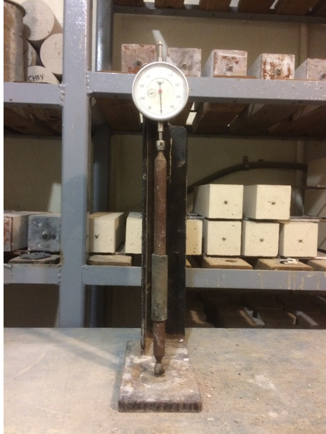
Figure 10: C157 testing apparatus for length change with the reference bar in place
