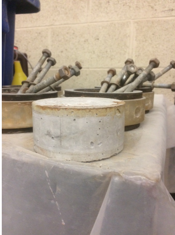
Figure 6: 2 in. (50-mm) tall cylinder used in RCIP testing cells
