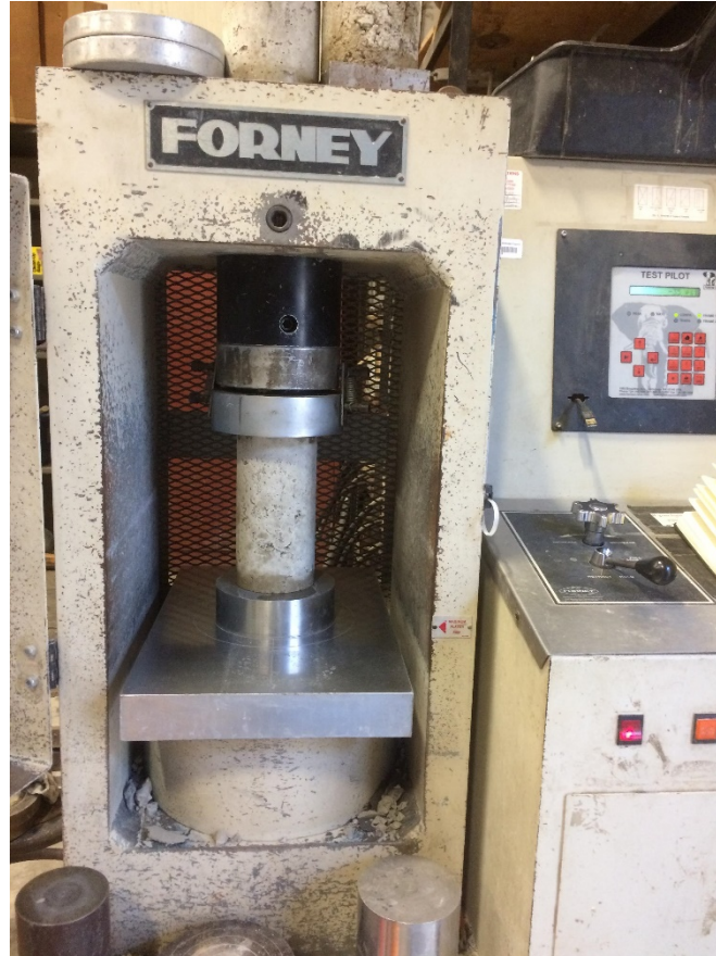
Figure 5: Forney machine used for compressive strength testing
