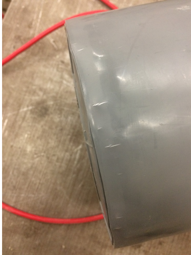
Figure 50: Visible expansion of the base with stretch marks on the mold for *ST210
