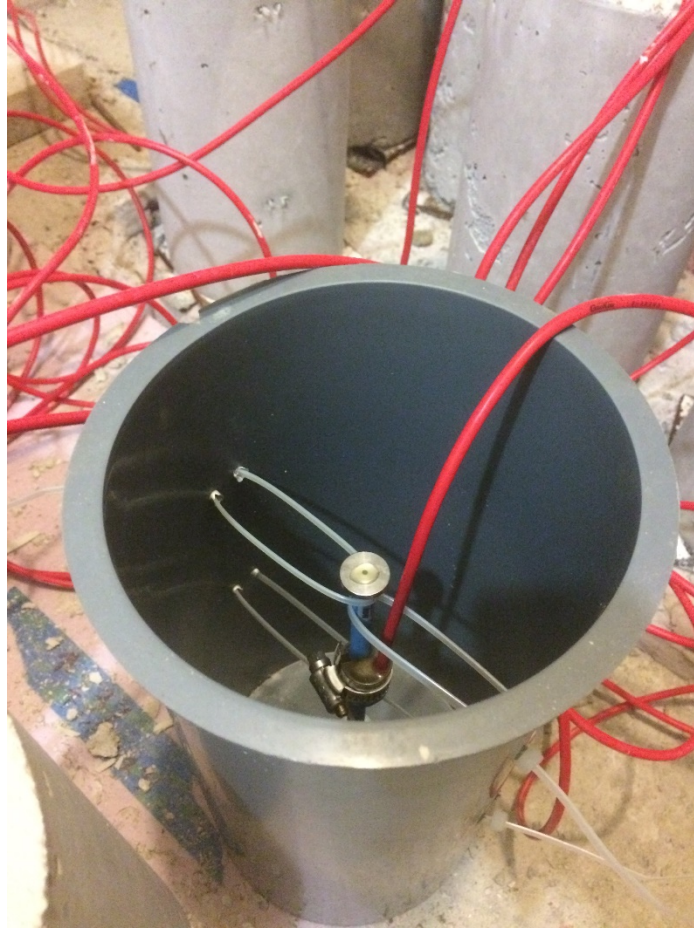
Figure 4: Geokon Model 4200 VW strain gage tied in cylinder prior to batching
