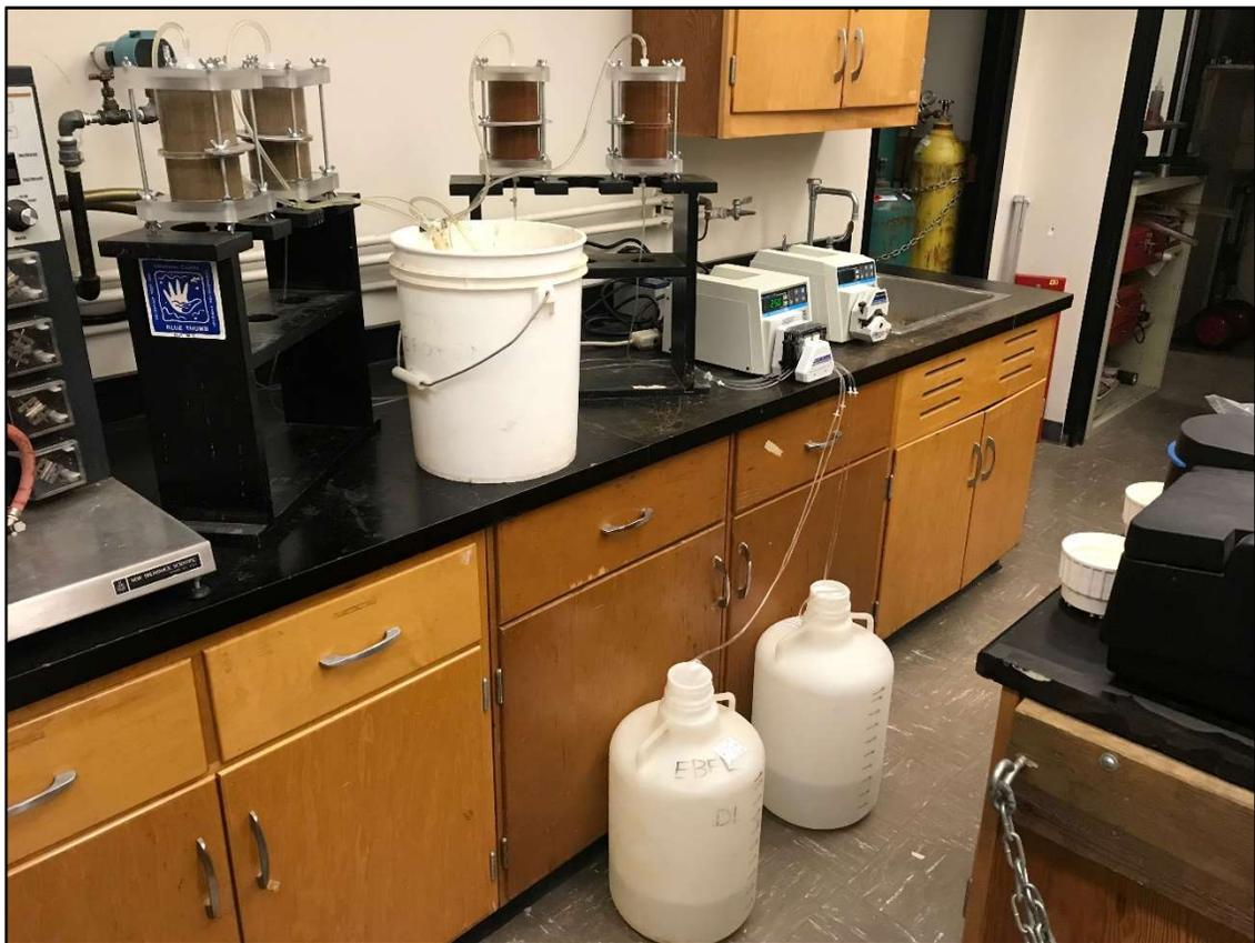
**Figure 5: Set-up of laboratory column experiments with synthetic stormwater sources in 20-L carboys, peristaltically pumped from bottom of packed columns (left: two FA5.0 columns; right: two MDR7.5 columns).**
